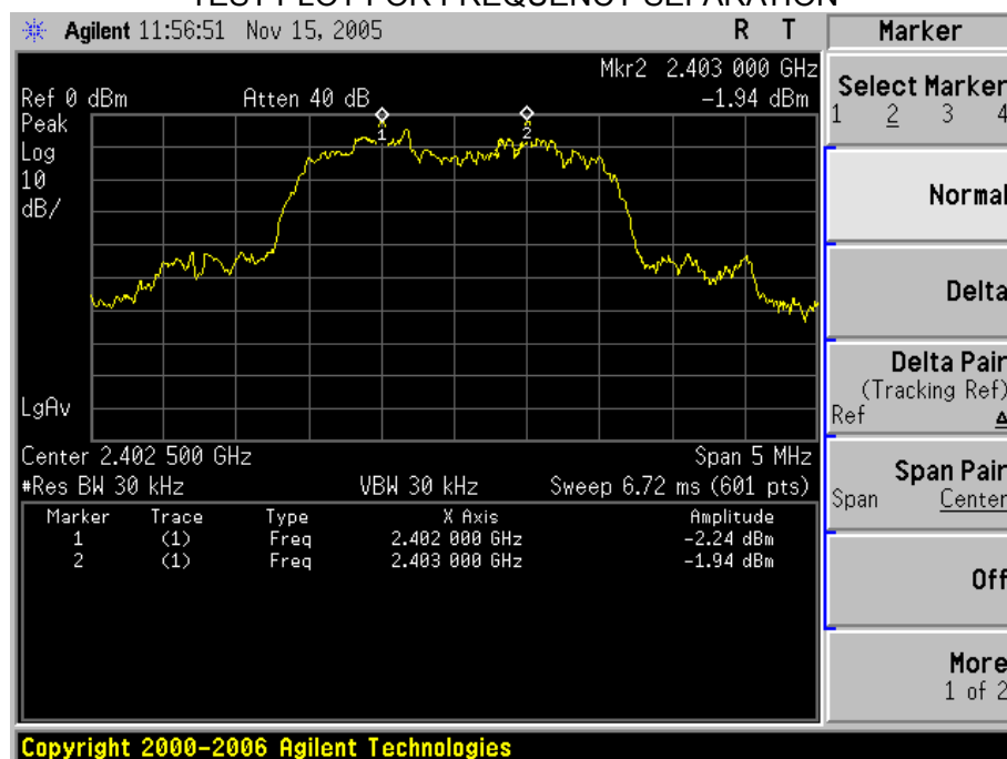
TEST PLOT FOR FREQUENCY SEPARATION
