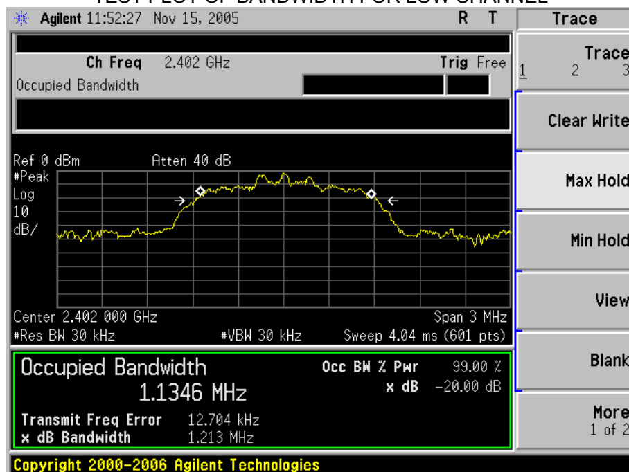
TEST PLOT OF BANDWIDTH FOR LOW CHANNEL
