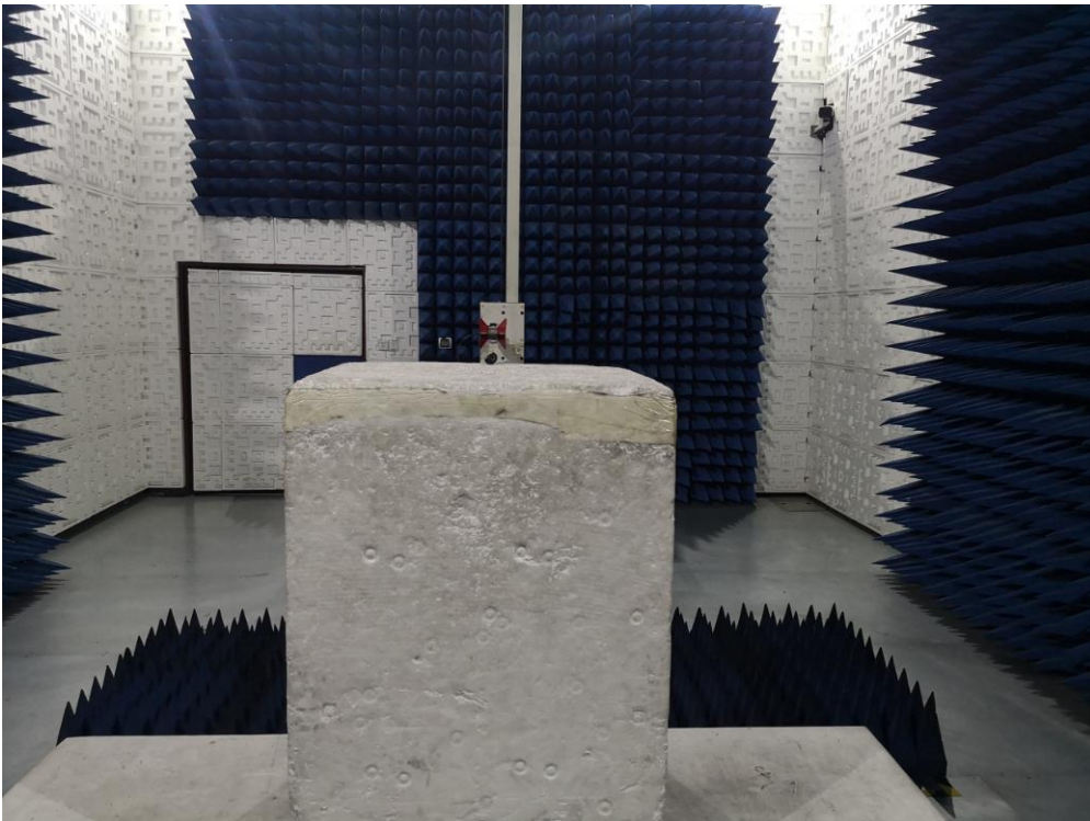
RADIATED EMISSION TEST SETUP ABOVE 1GHz
