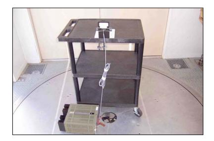
**Test Conditions:** EUT is a multi-technology reader operating on a frequency of 13.56MHz. EUT is mounted on a vertical support structure, simulating normal installation. DC power is provided via support power supply. Power supply is bonded to ground plane.
