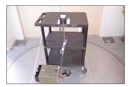
**Test Conditions:** EUT is a multi-technology reader operating on a frequency of 125kHz and 13.56MHz. EUT is mounted on a vertical support structure, simulating normal installation. DC power is provided via support power supply. Power supply is bonded to ground plane.
