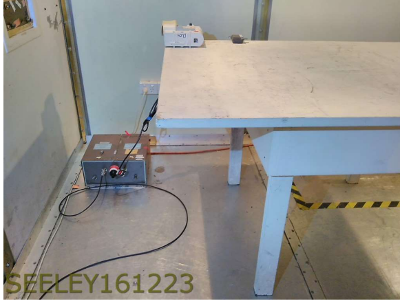
Mains Conducted Emissions -Wireless Receiver
