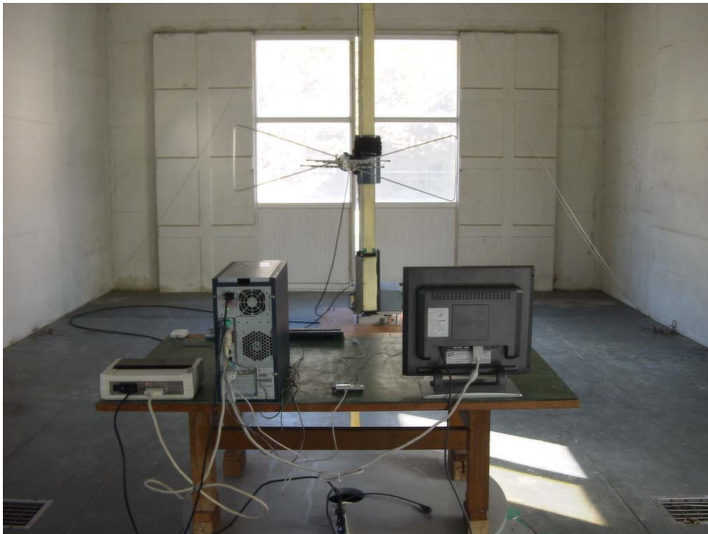
Radiated Emissions (File up/download mode) - Rear View
