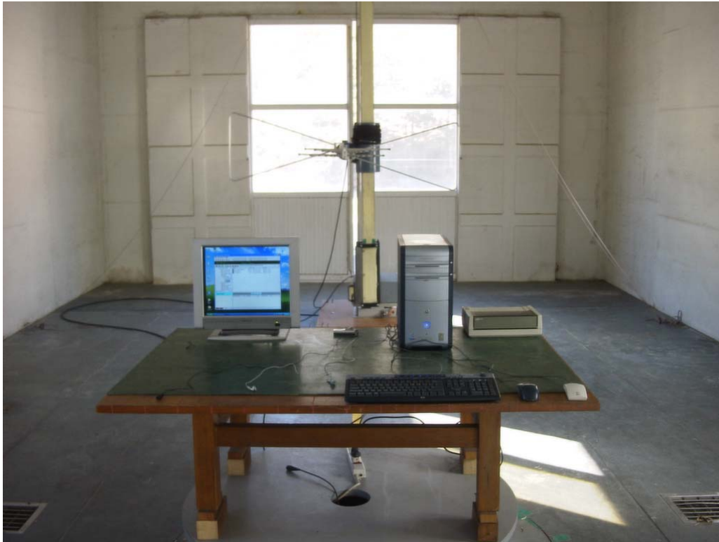
Radiated Emissions (File up/download mode) - Front View
