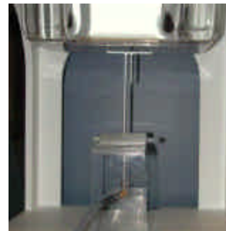
Figure A.0 Dipole Validation Test Setup
