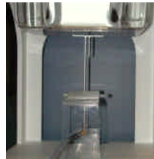
Figure A.0 Dipole Validation Test Setup
