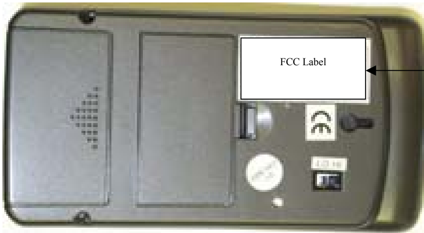
Figure 2.2 FCC ID Label Location
