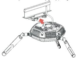
10. If the access point is not properly secured, press the release button on top of the bracket to unlock the access point. Making sure that the cable is still connected, repeat Steps 8 and 9.
