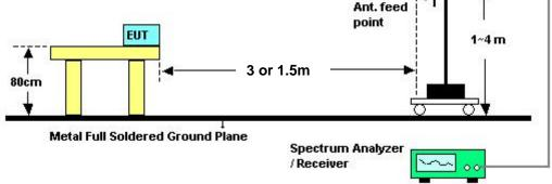
Above 5GHz shall be extrapolated to the specified distance using an extrapolation factor of 20 dB/decade form 3m to 1.5m.
