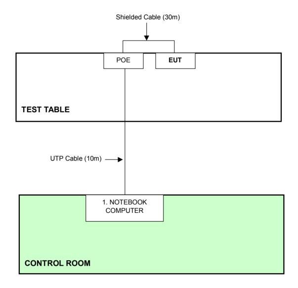
**NOTE:** 1. Support unit 1 was kept in the control room during the test.
