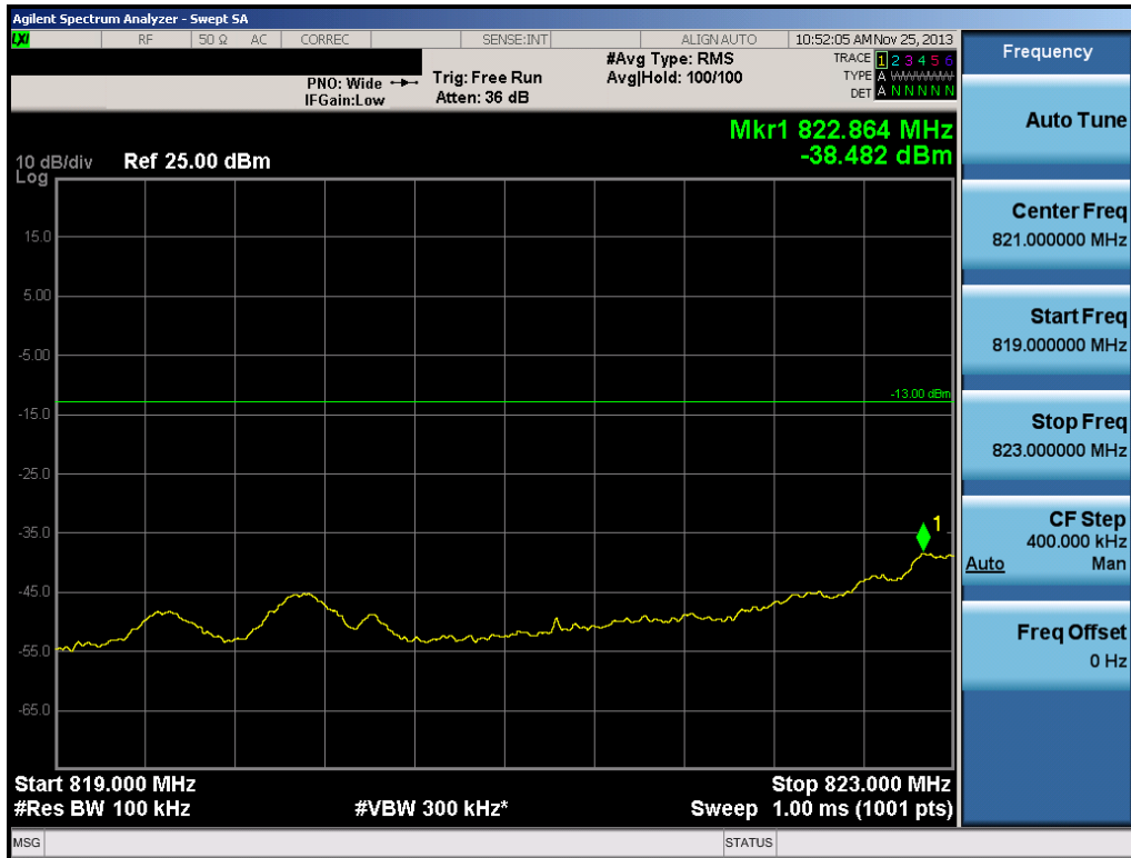
Plot 6-16. 4MHz Span Plot (Cellular CDMA Mode – Ch. 1013)
