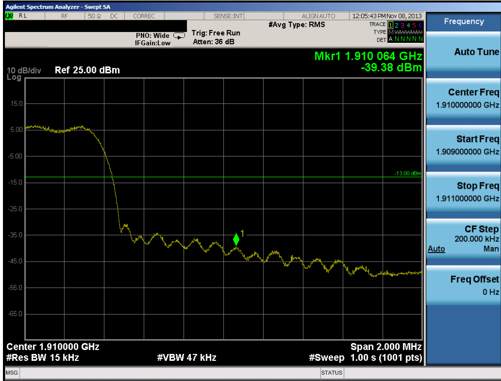
Plot 6-21. Band Edge Plot (PCS CDMA Mode – Ch. 1175)
