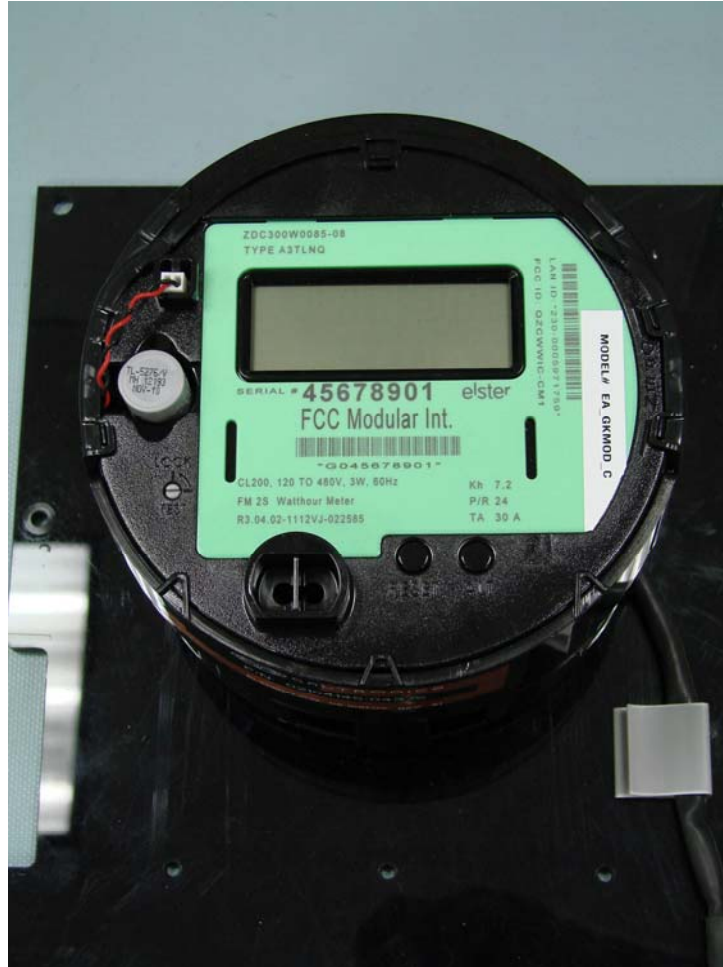
Modular EA_Gatekeeper with internal antennas completed assembly
