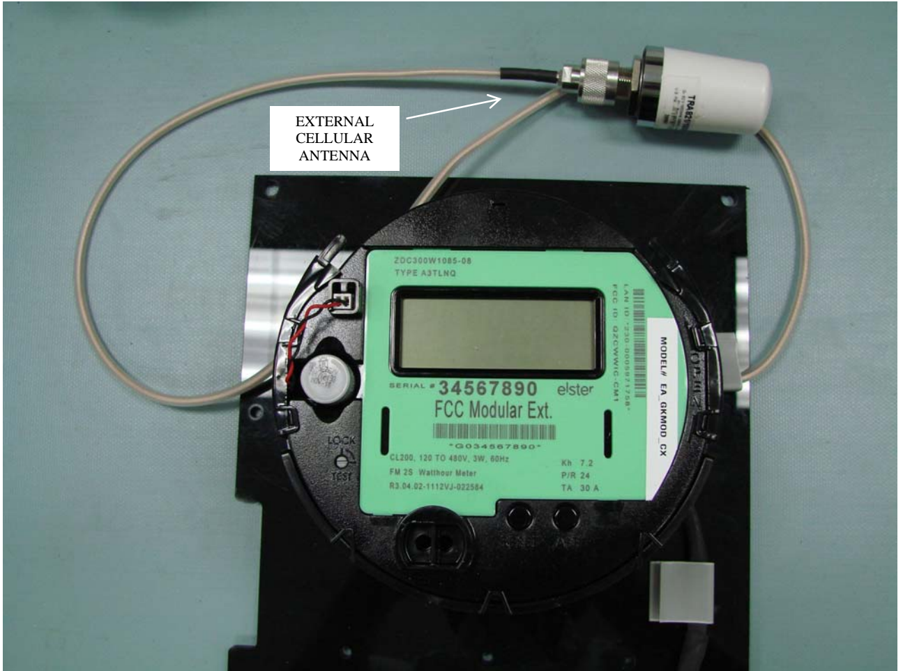
Modular EA_Gatekeeper with internal ISM/external cellular antennas completed assembly
