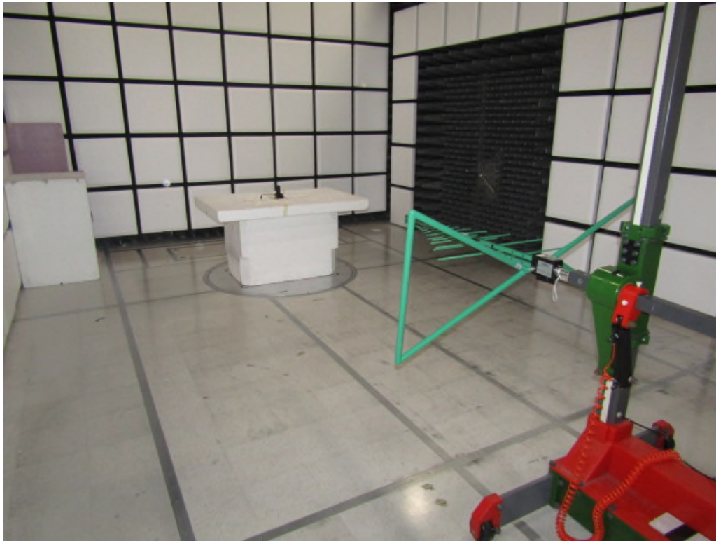
Figure 1: Radiated Emissions – Front – Below 1GHz – Form Factor 1
