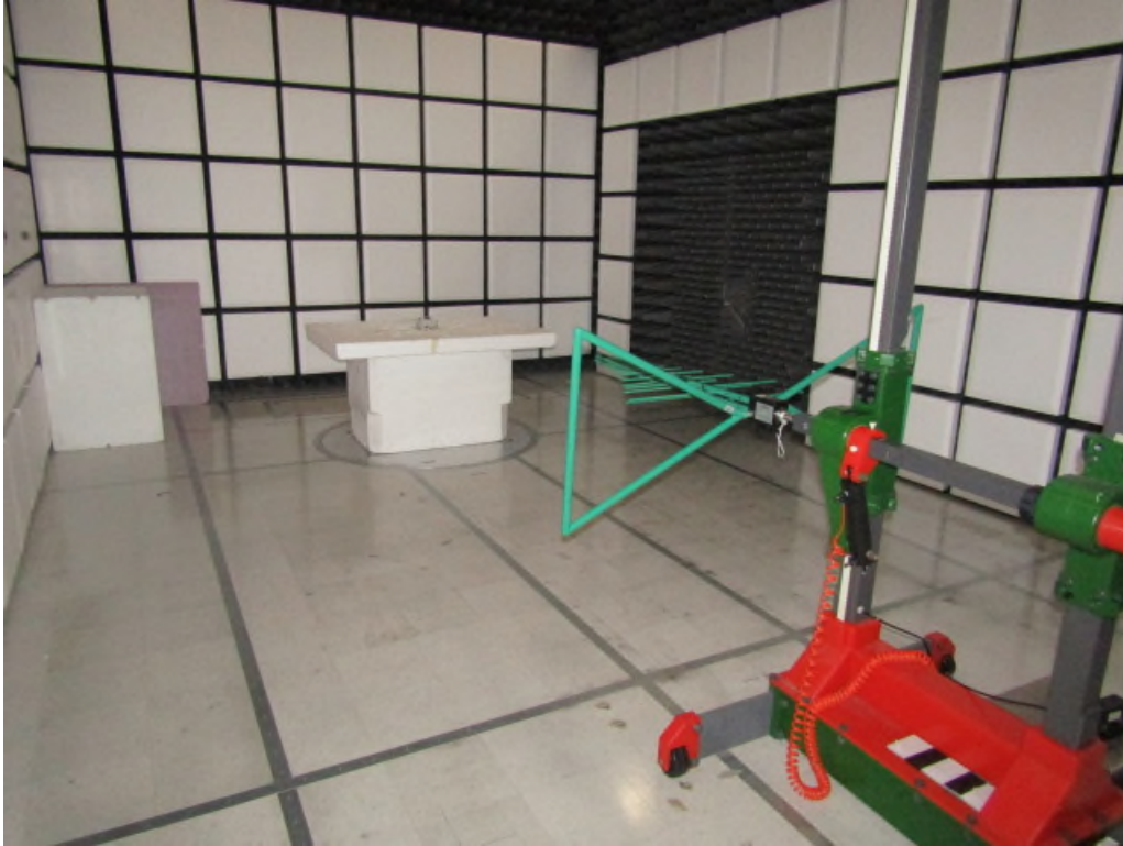
Figure 3: Radiated Emissions – Front – Below 1GHz – Form Factor 2
