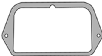
Type S Angled lens with a single screw groove at the top and two screw holes on the sides.
