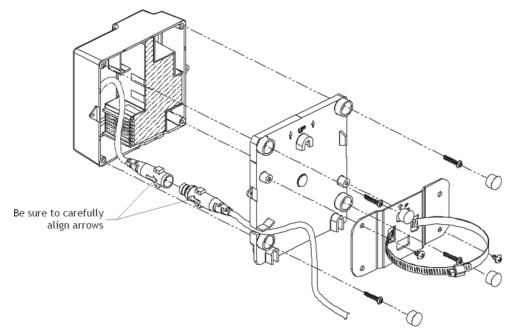
4 Insert the cable back into the Honeywell Water 4.0 module, making sure to provide strain relief for the cable. Be sure to securely fashion the cable by using the cable tie as illustrated in the next figure.
