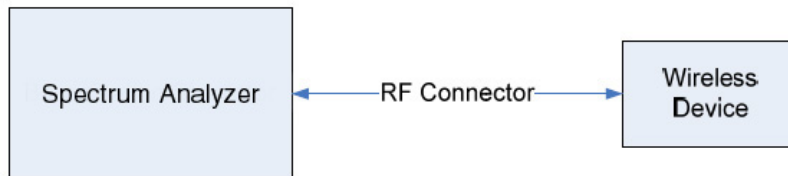
Figure 6-2. Test Instrument & Measurement Setup
