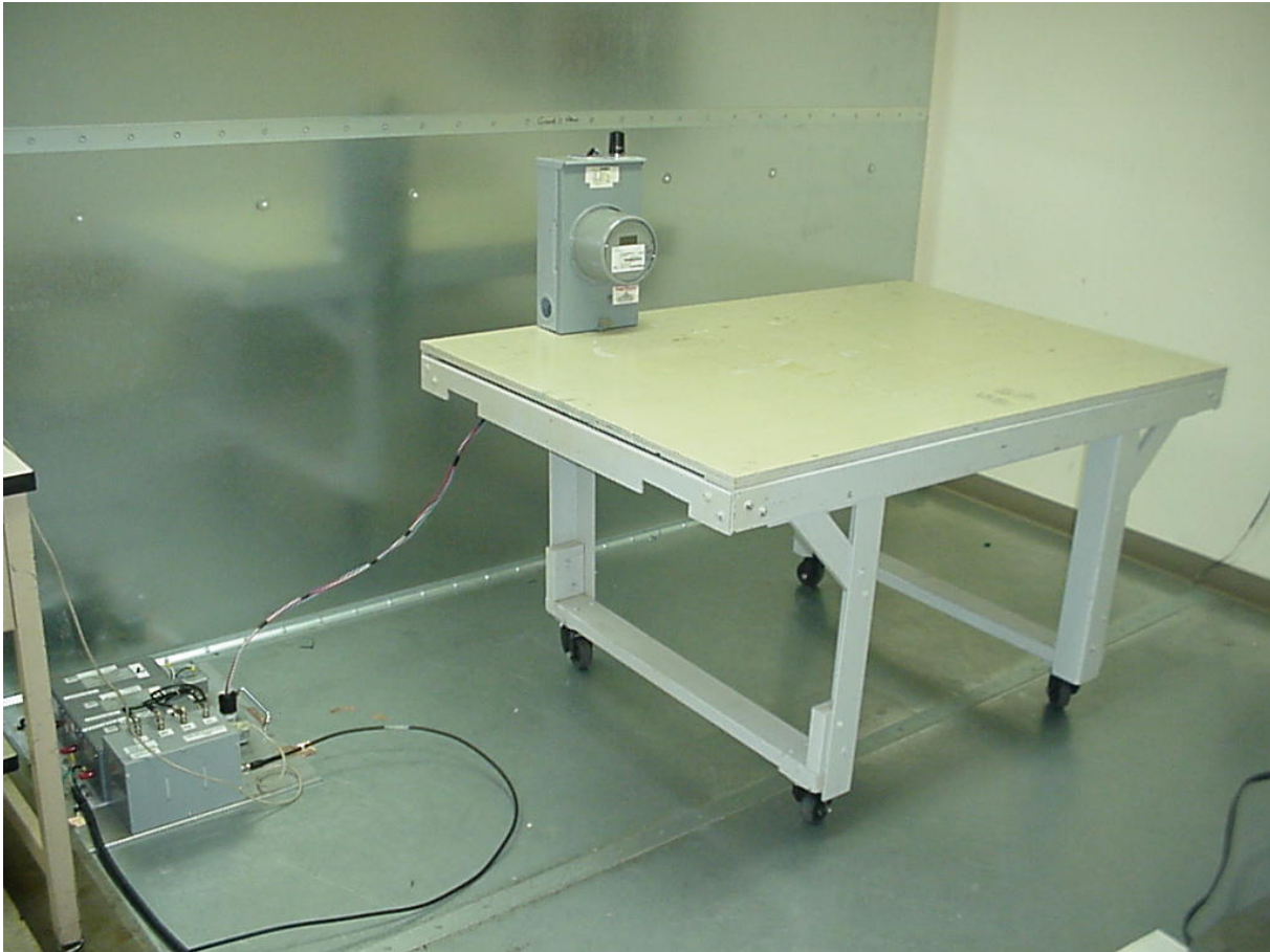
Figure 9 - Conducted Emissions Test Setup (Front)
