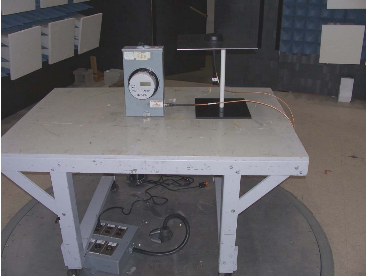
Front View of Test Setup with the Larsen LP800NMO Antenna
