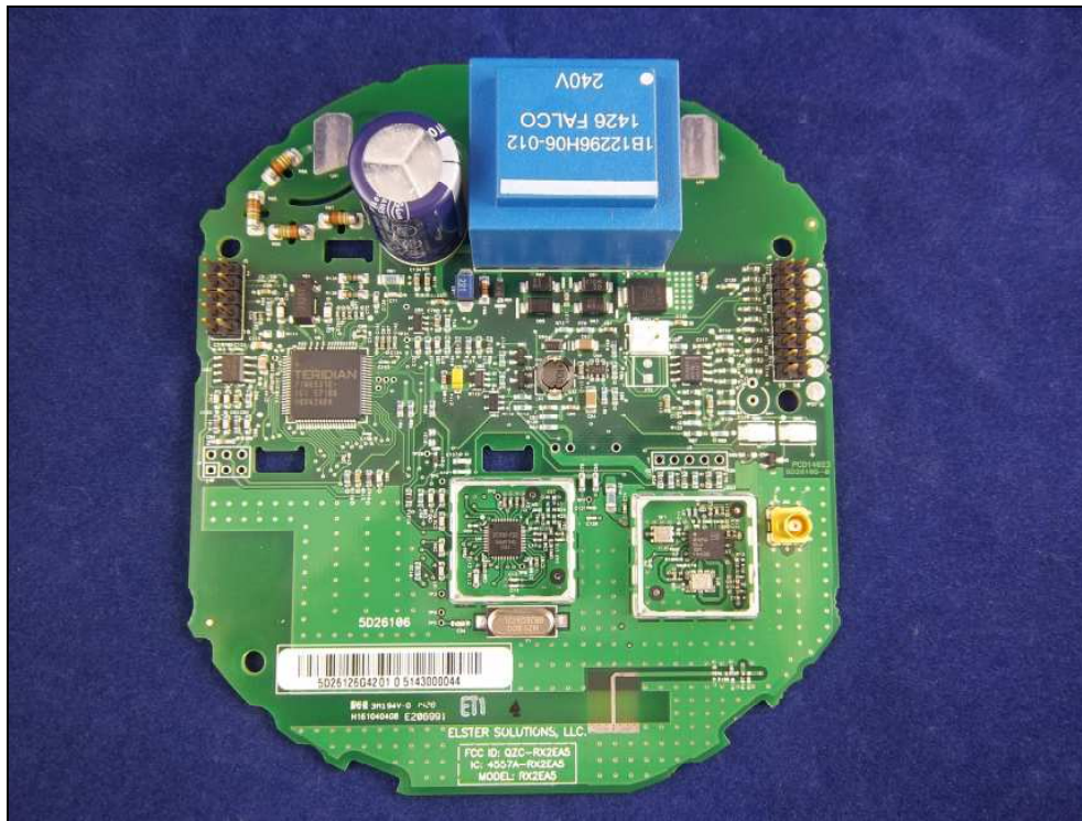
Figure 5: Internal Photo – Shields Removed
