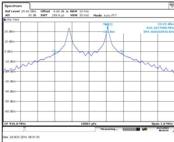
Figure 7.4.4.2.5: 99% BW Mid Channel
