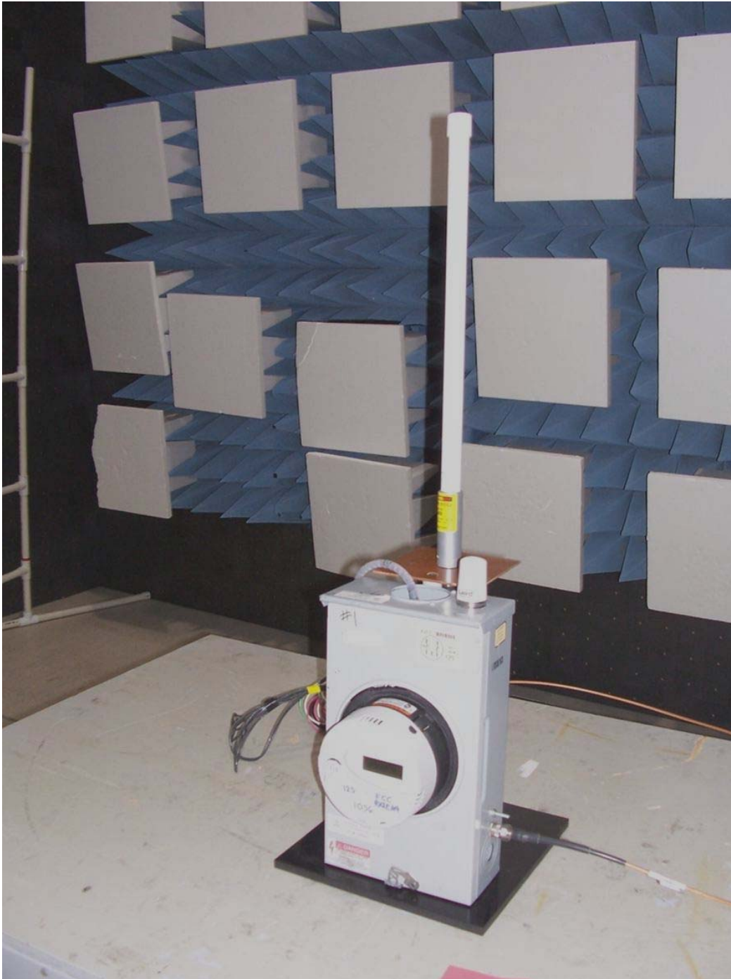
Front View of Test Setup with the highest gain External Antenna.
