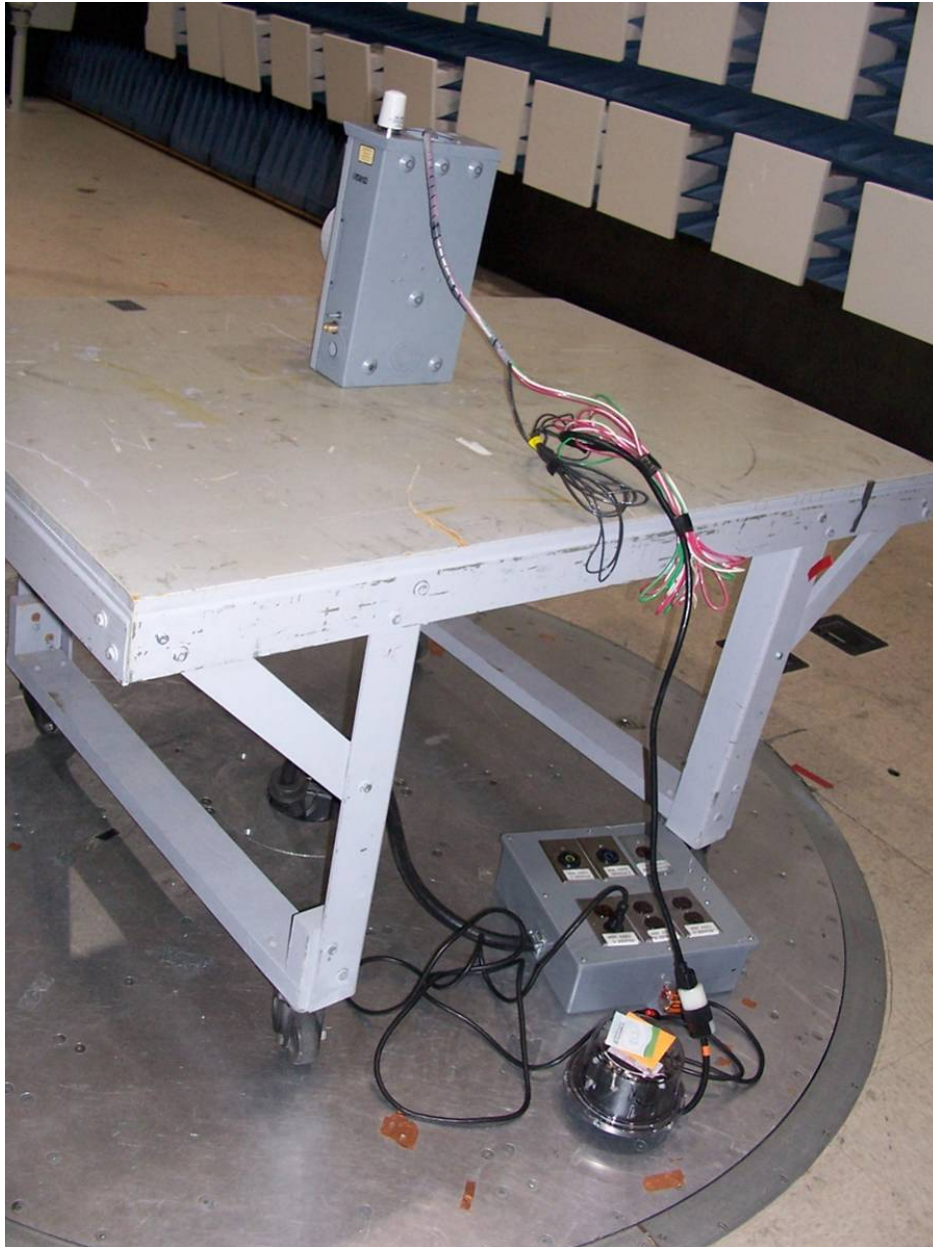
Rear View of Test Setup with the Internal Antenna
