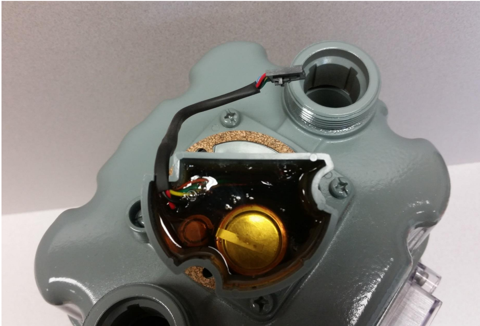
The battery and supercapacitor are visible through the bottom of the potting cup.
