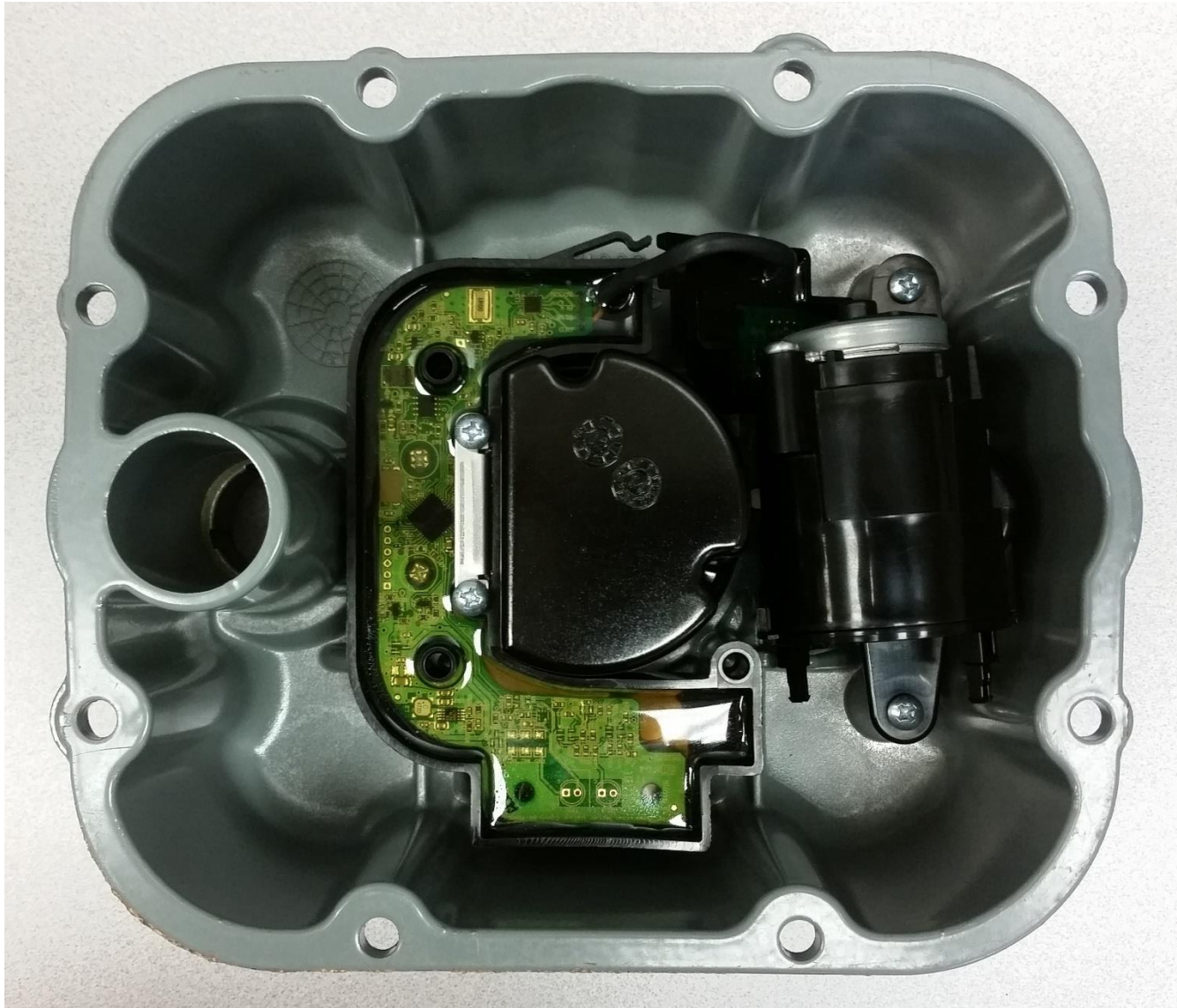
The inside of the meter top contains a gas valve (right) and the valve control electronics.
