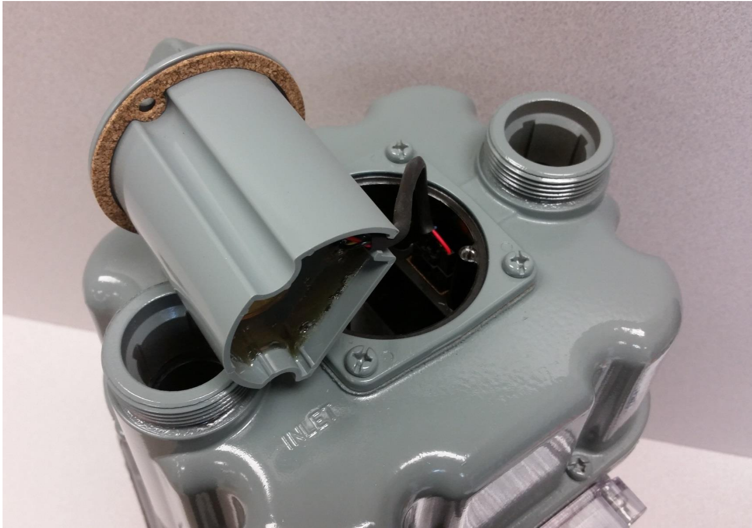
The potting cup is shown removed from the rest of the meter, but still connected via its wire harness. The potting cup contains the radio transceiver, battery, and supercapacitor.
