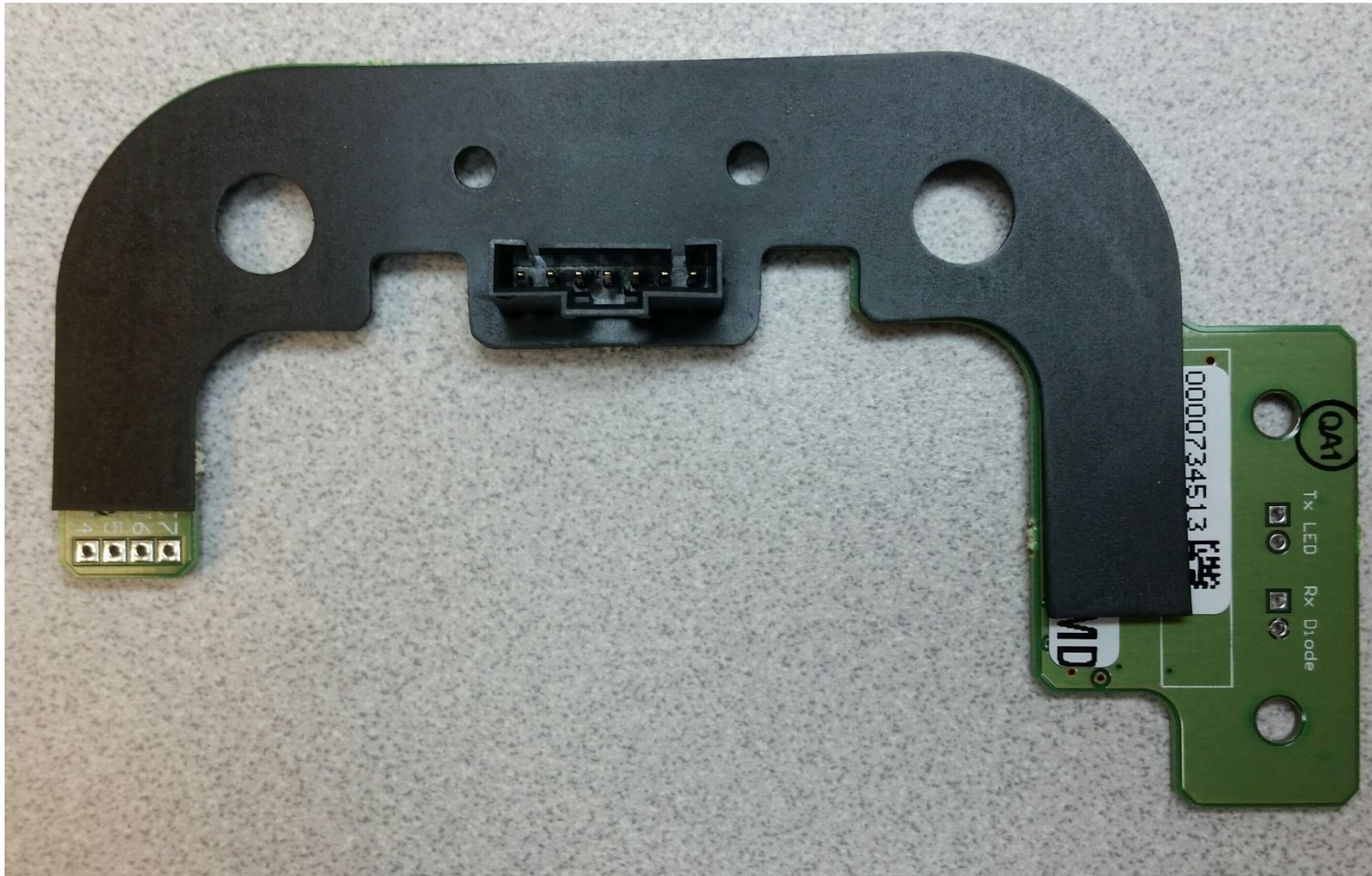
Back side of the valve control module. There are no electronic parts on this side of the board, other than the 7-pin connector shown.
