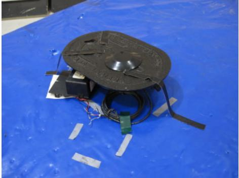
Note: Attaching wires are coiled in water meter housing per manufacturer's instructions. Larger battery used for test is placed as closely under perimeter of the lid as possible to best represent and installation arrangement.
