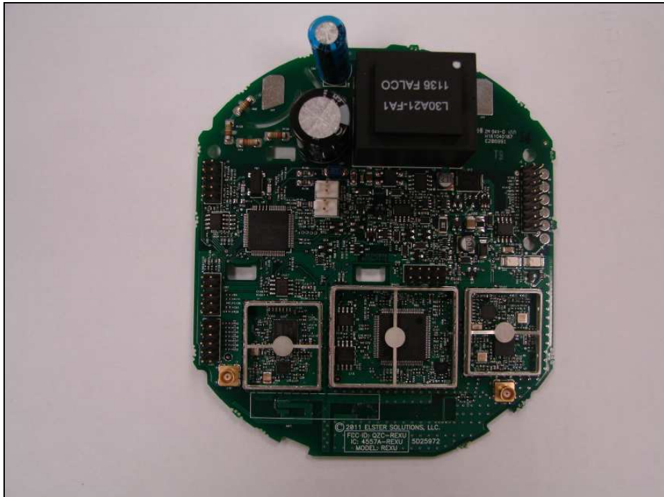
Figure 1: Internal Photo – Shields Removed
