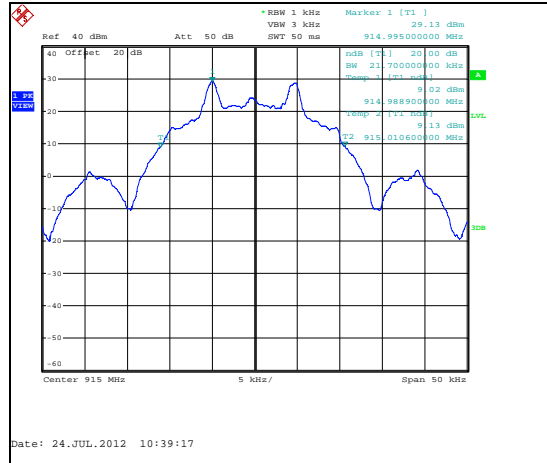
Figure 7.4.4.2-26: 20dB BW - 915.0 MHz – 9.6 kbps
