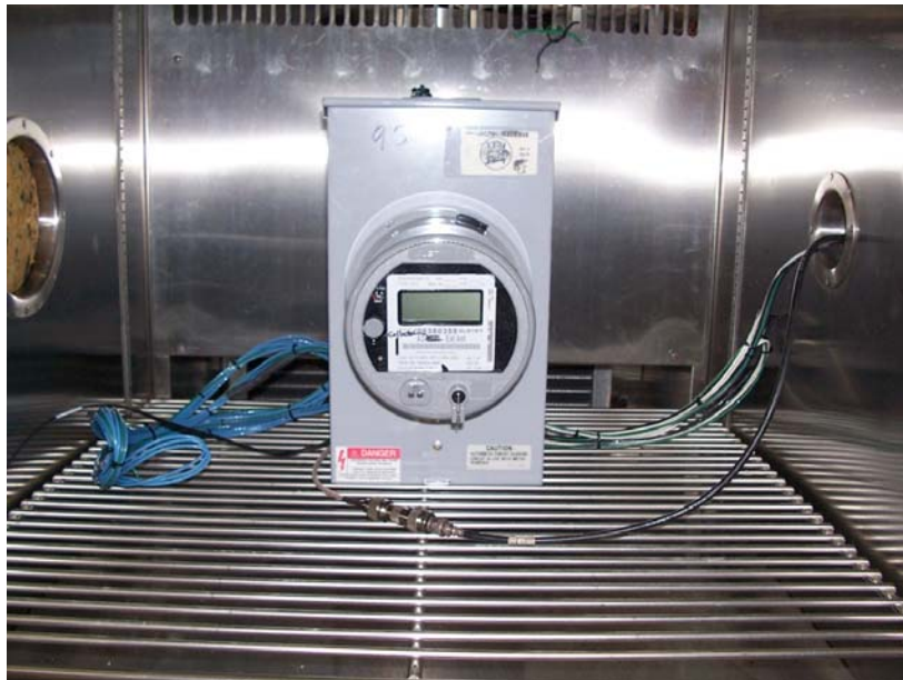
Photo of Frequency Stability over temperature variations test.
