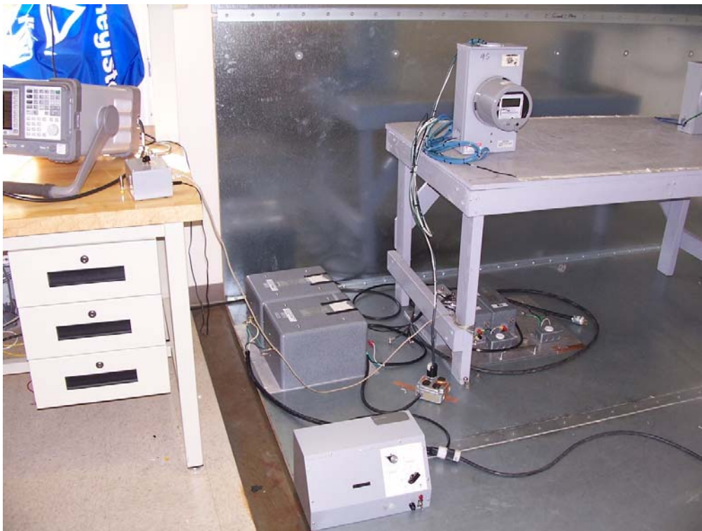
Photo of Conducted Emission of EUT Model No. ZD3200K20xx with External Antenna adapter
