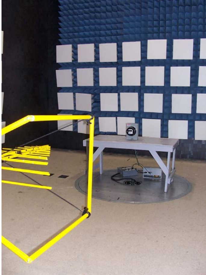
Photo of Radiated and Spurious Emissions Measurements
