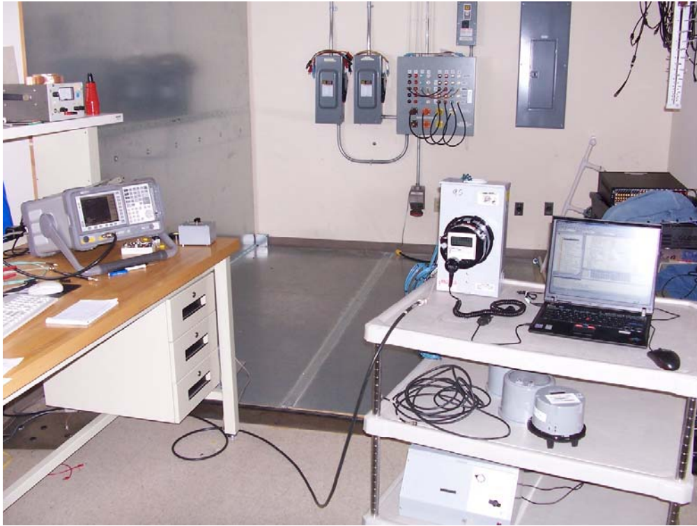
Photo of Setup for Channel separation, time of occupancy occupied bandwidth and Peak power measurements. Also frequency stability over voltage variations using adjustable transformer located on bottom of cart.
