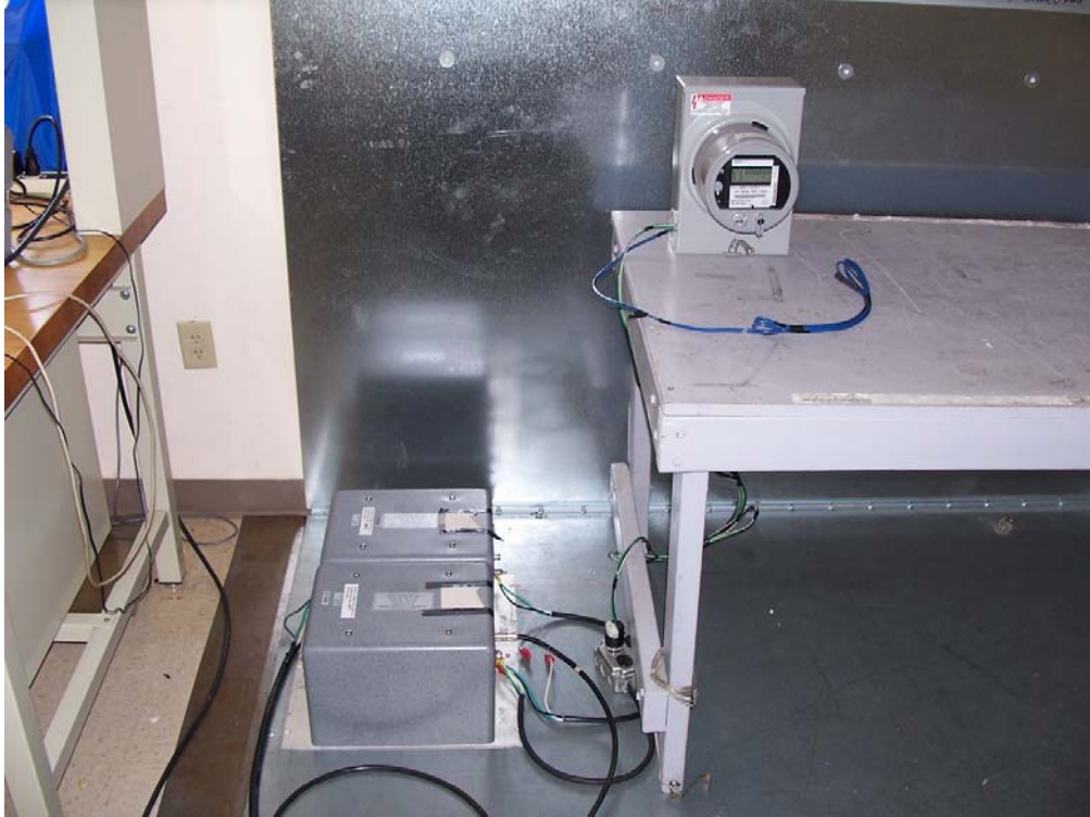
Photo of Conducted Emission of EUT Model No. ZDC300K00xx with Internal Antenna
