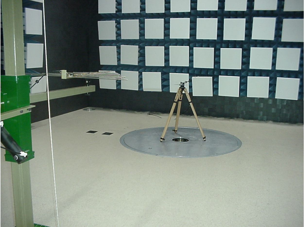
Setup for Substitution Method
