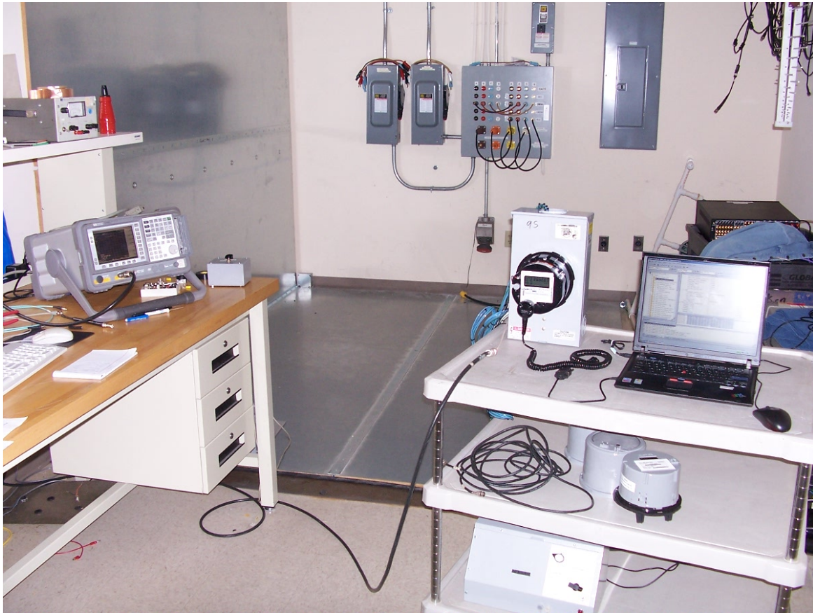
Figure 11 – Setup for Conducted Power Measurements
