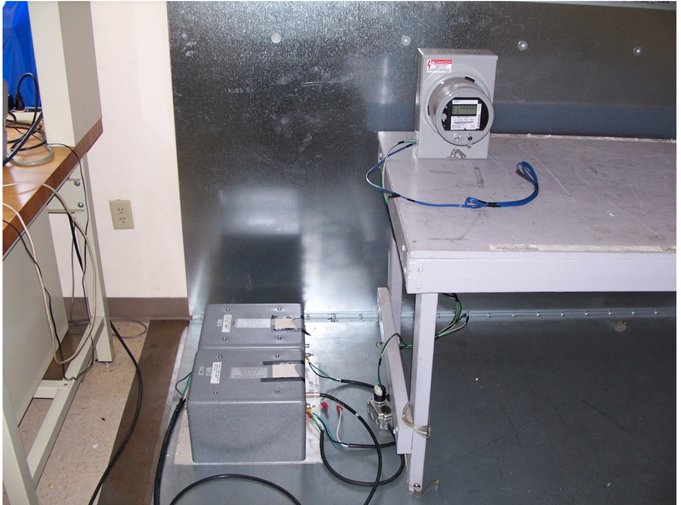
Figure 12 - Conducted Emissions Test Setup (Front)
