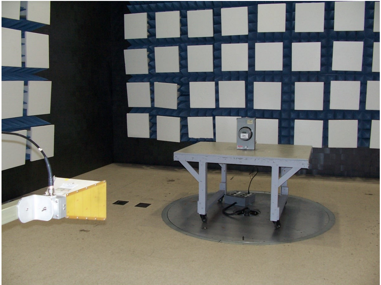
Figure 8 - Radiated Emissions Test Setup (Chamber – Back, X orientation)
