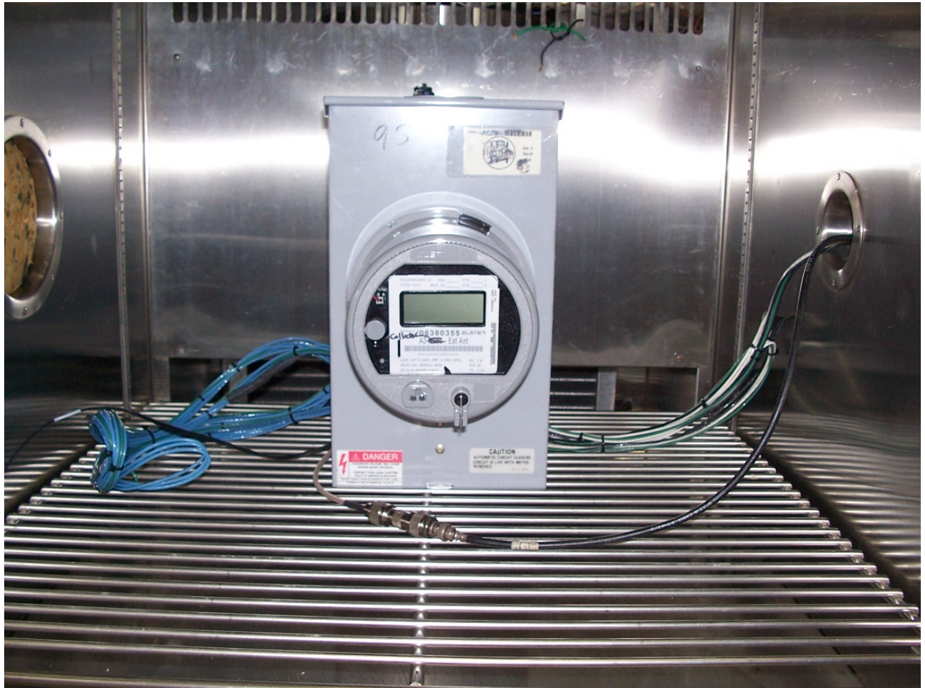
Figure 9 – Temperature Chamber Setup
