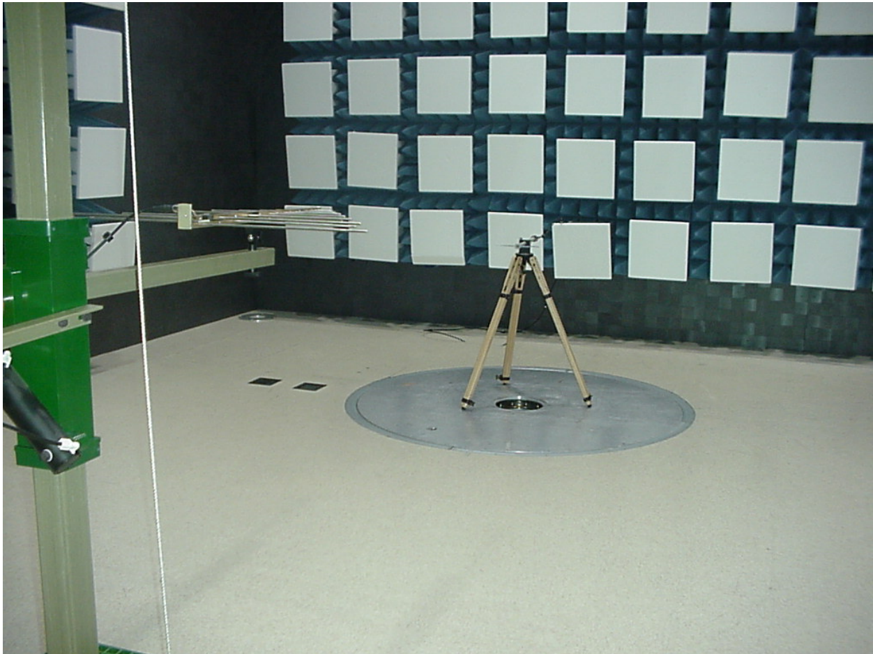
Figure 10 – Setup for Substitution Method
