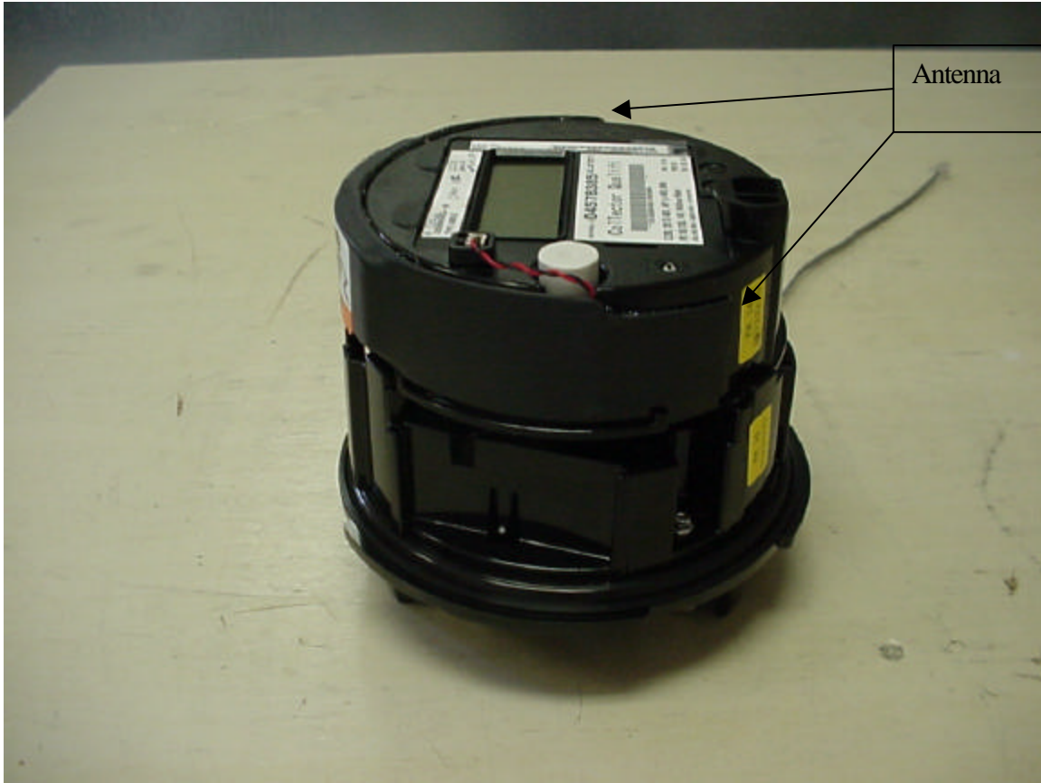
EUT with outer shell removed.
