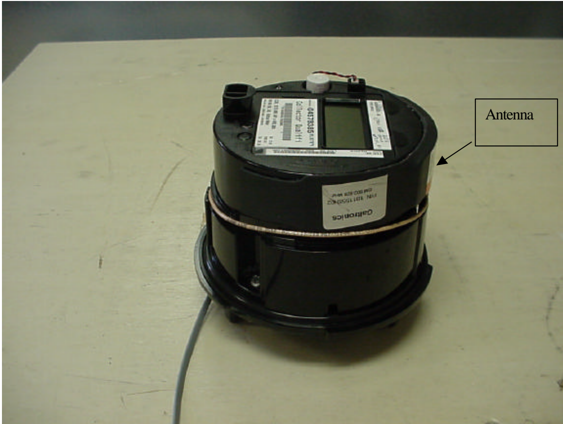
EUT with outer shell removed.
