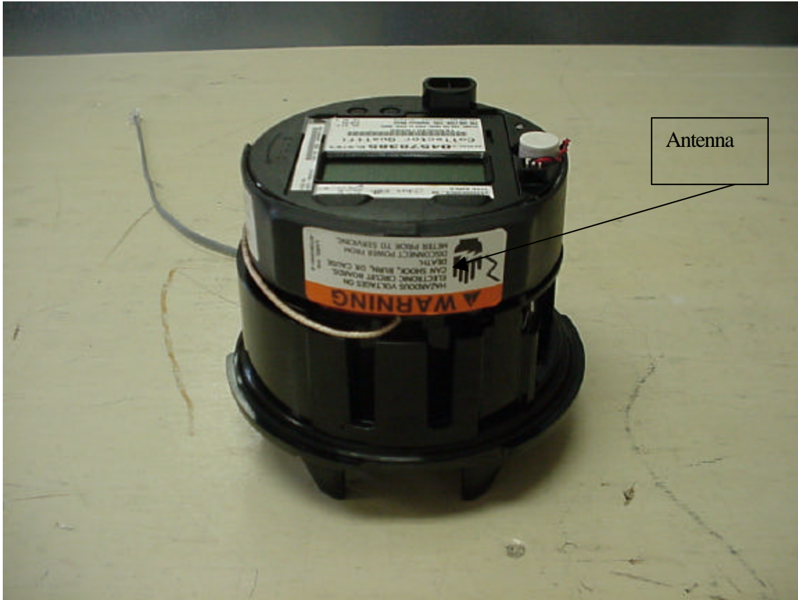
EUT with outer shell removed.
