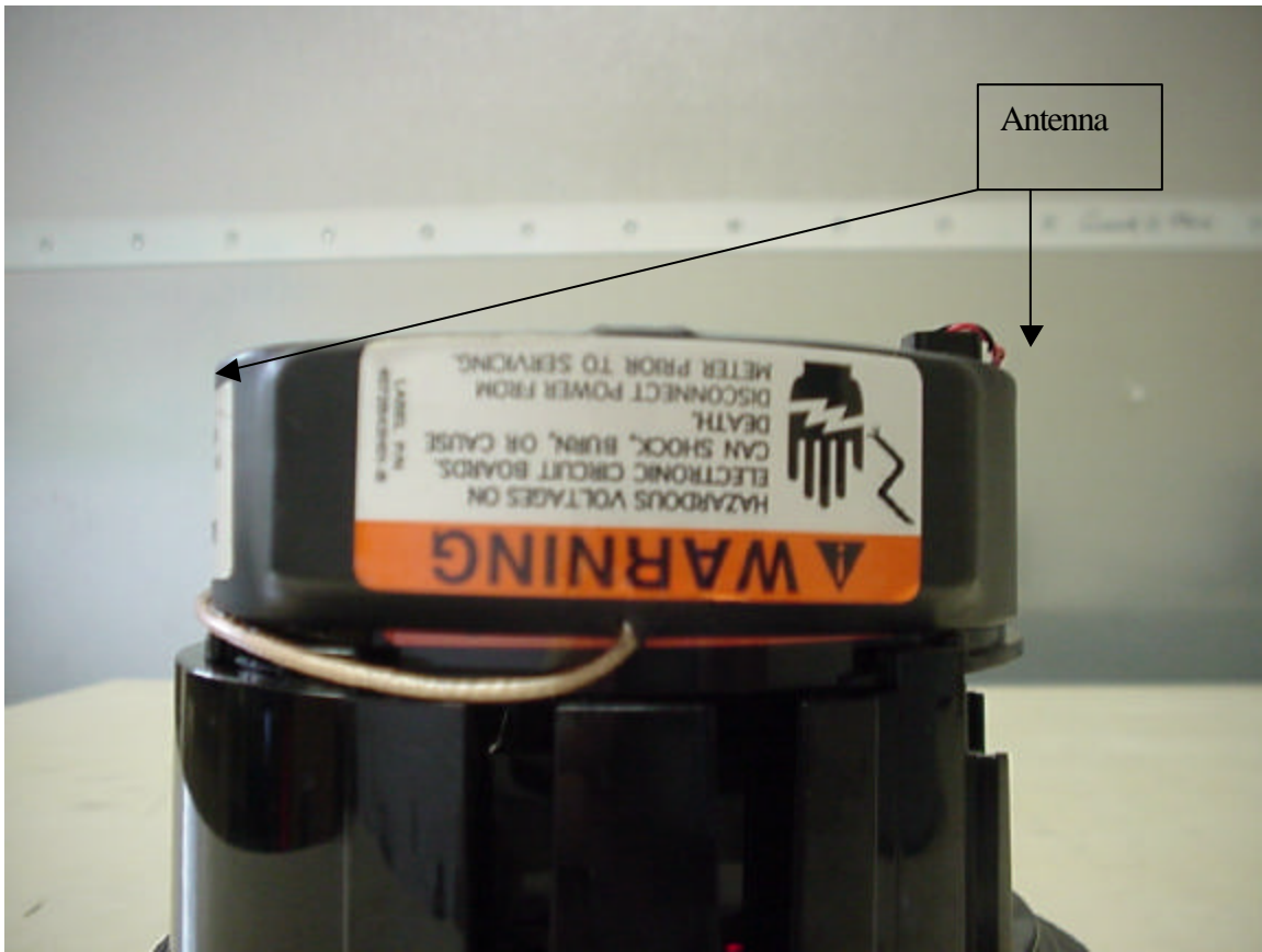
EUT with outer shell removed.
