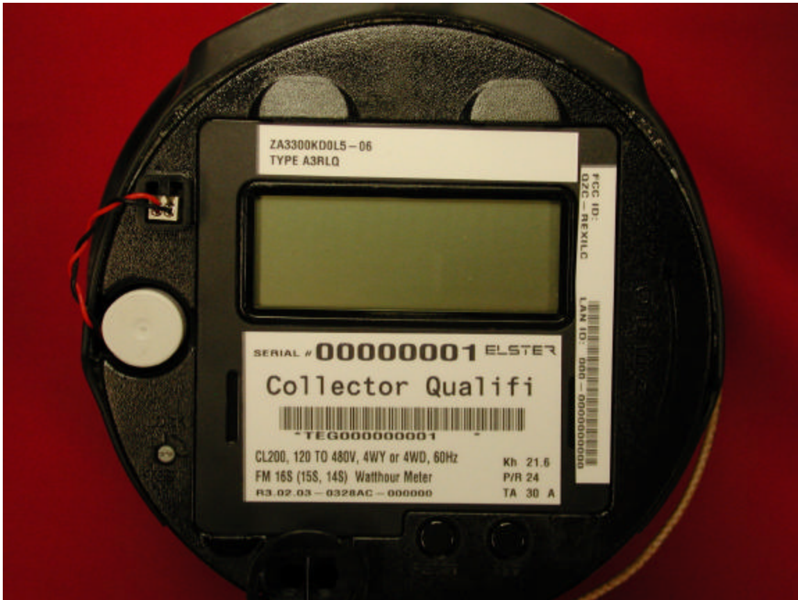
Figure 1: A3 Collector Nameplate
