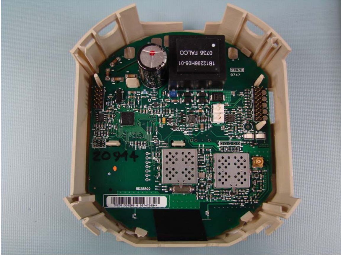
INTERNAL ASSEMBLY SHOWING PCB INSTALLED IN FRONT COVER
