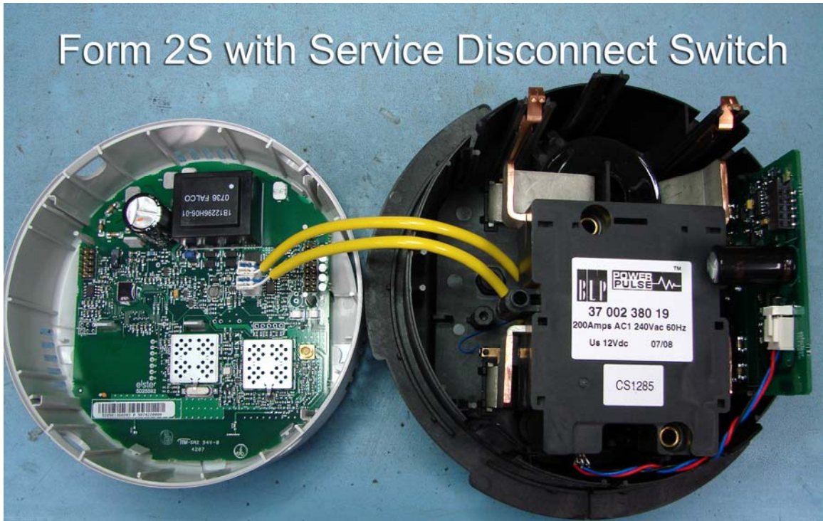
INTERNAL ASSEMBLY VIEW FORM 2S WITH SERVICE DISCONNECT SWITCH
