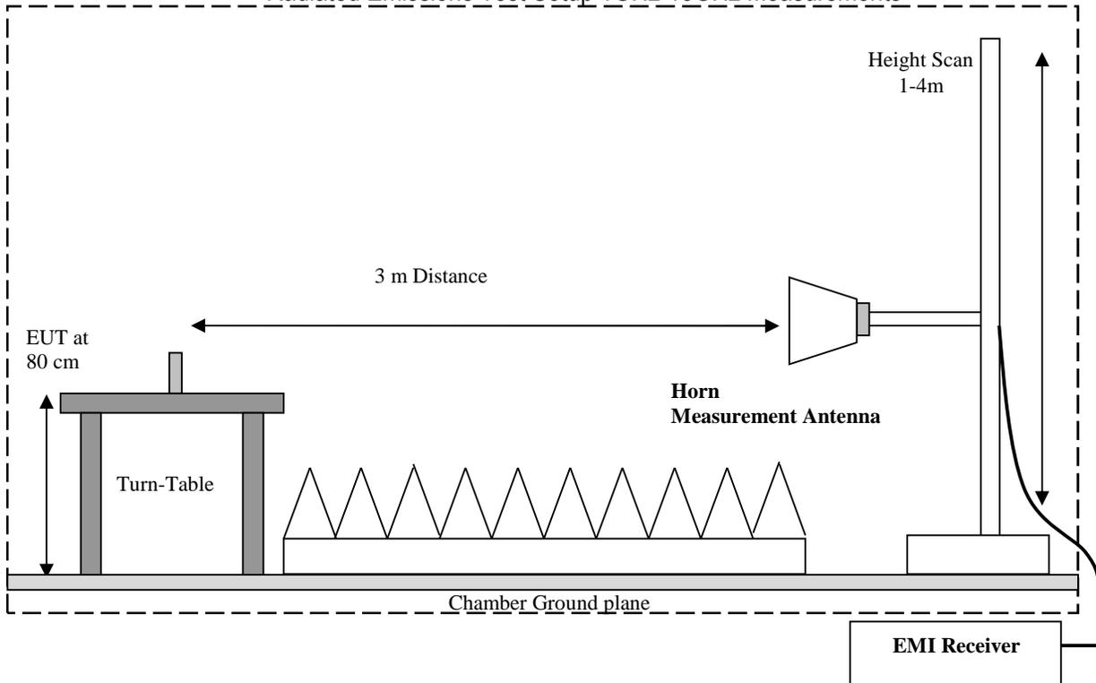
Radiated Emissions Test Setup 18GHz-40GHz Measurements
