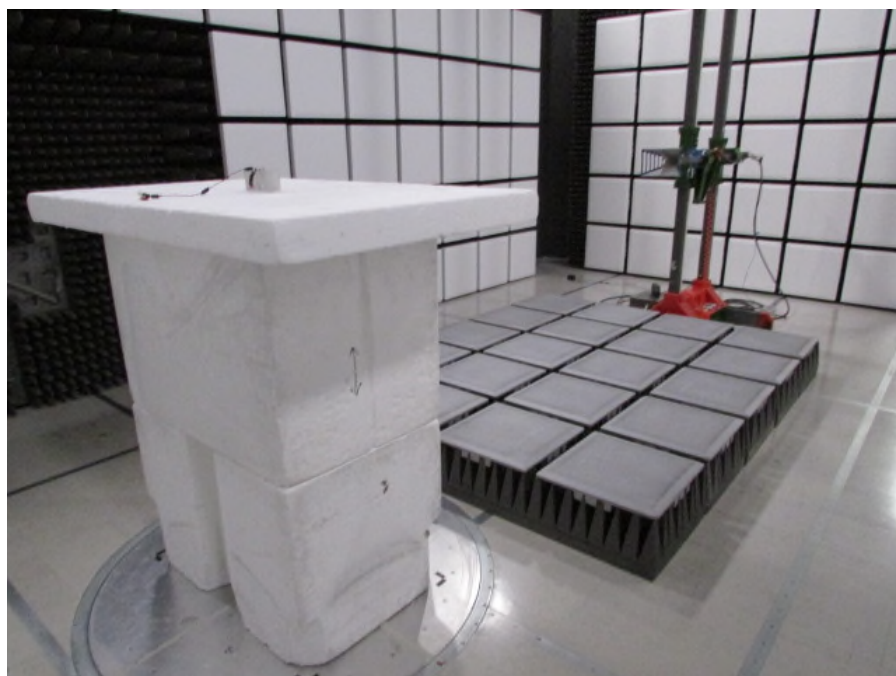
Figure 7: Radiated Emissions – Back – Above 1GHz
