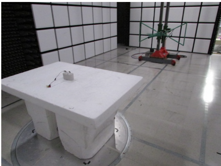
Figure 2: Radiated Emissions – Back – Below 1GHz
