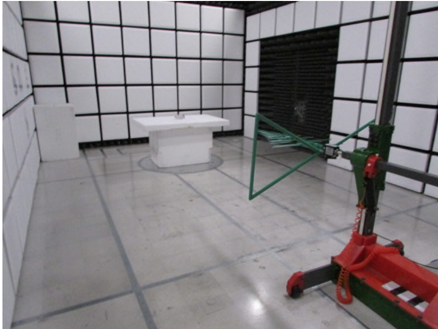
Figure 1: Radiated Emissions – Front – Below 1GHz
