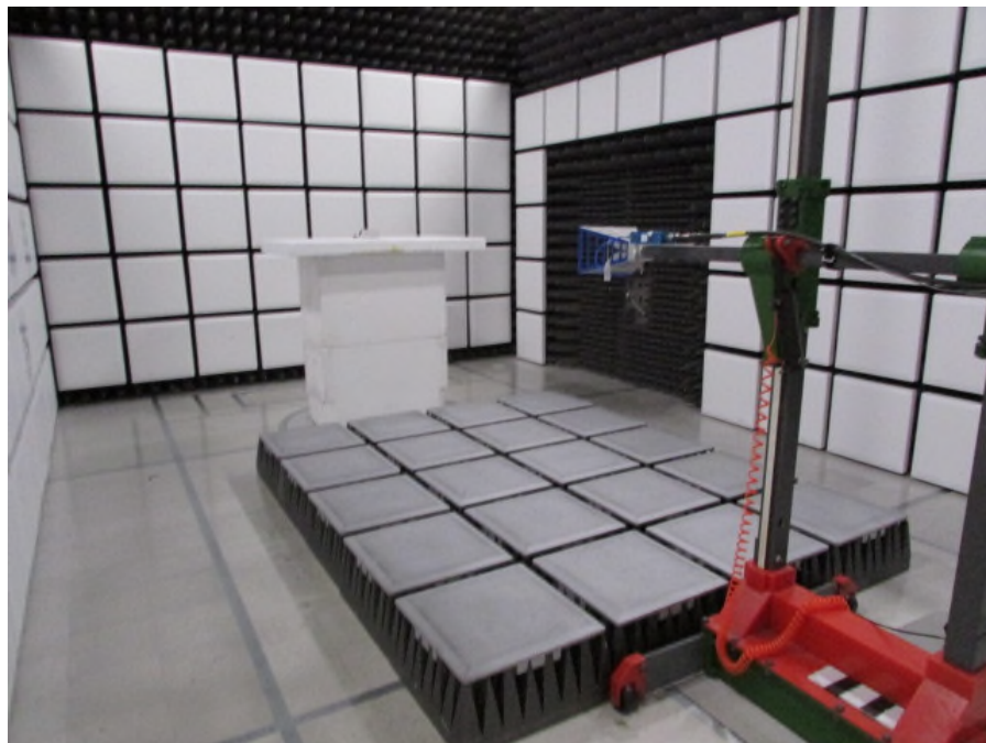
Figure 6: Radiated Emissions – Front – Above 1GHz
