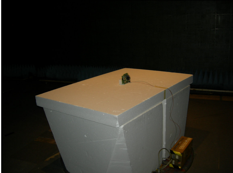
Figure 2: Radiated Emissions – Internal Antenna
