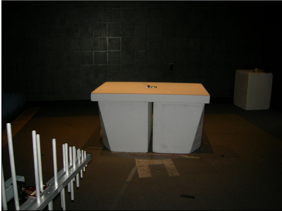
Figure 1: Radiated Emissions – Internal Antenna
