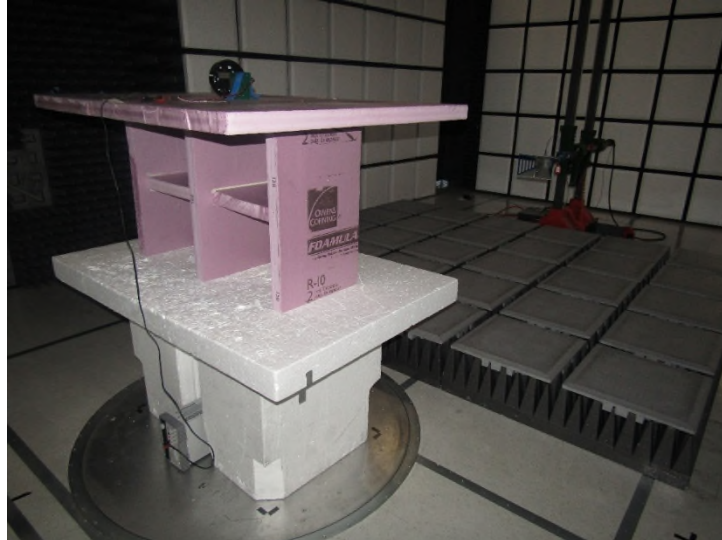
Figure 8: Radiated Emissions – Above 1 GHz (Inverted F Antenna) – Rear View
