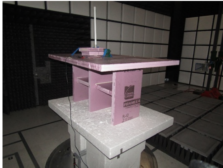
Figure 6: Radiated Emissions – Above 1 GHz (Half-Wave Dipole Antenna) – Rear View
