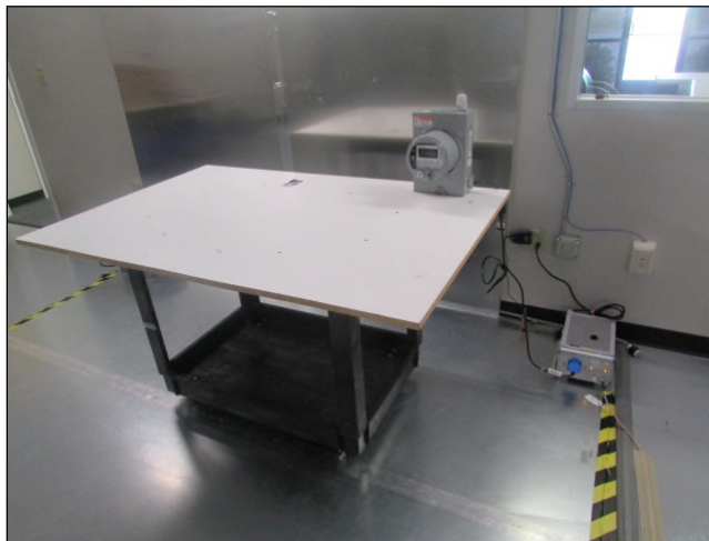
Figure 1: Power Line Conducted Emissions – Front View
