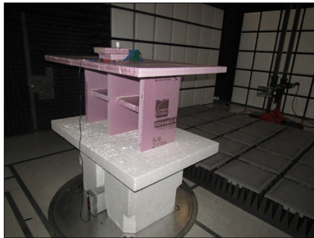
Figure 4: Radiated Emissions – Above 1 GHz (Spiral Antenna) – Rear View
