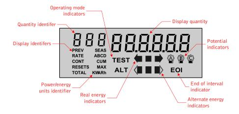
The display list for all displayable items, including the items relating to the ILC2 option board, can be programmed using Metercat meter support software.
