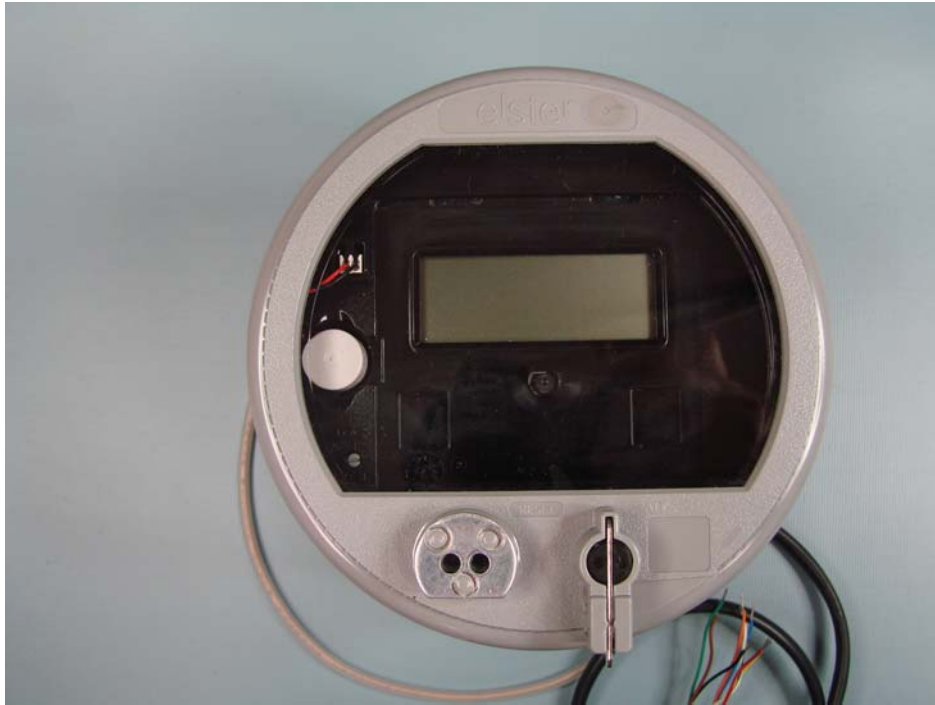
Host A3 Meter Exterior Front View
