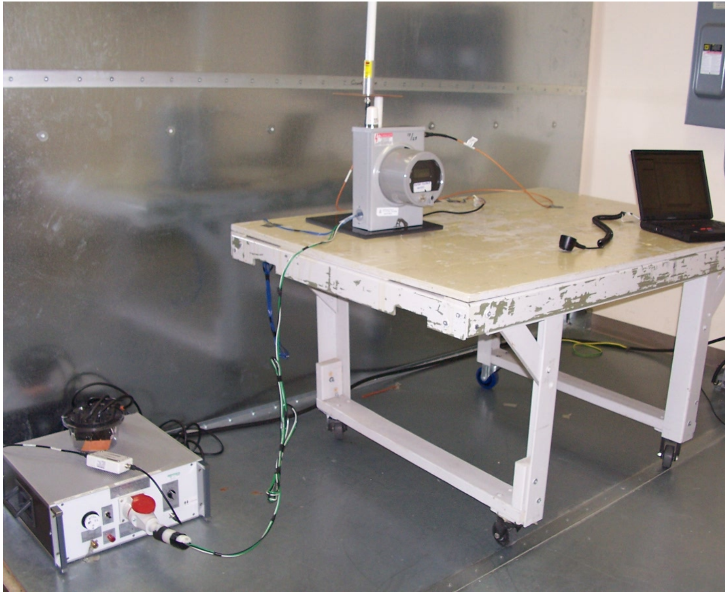
View of Test Setup for Conducted Emissions on AC Mains EUT using the External Antenna
