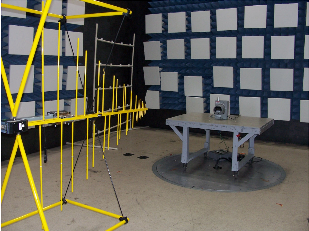
Typical View of Test Setup for Radiated Emissions from 30 MHz to 1 GHz
