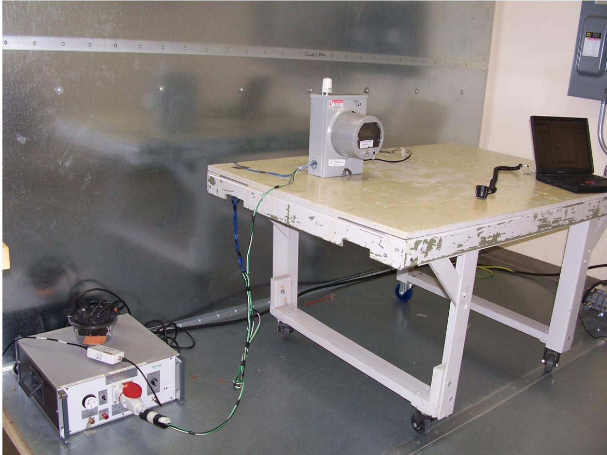
View of Test Setup for Conducted Emissions on AC Mains EUT using the Internal Antenna
