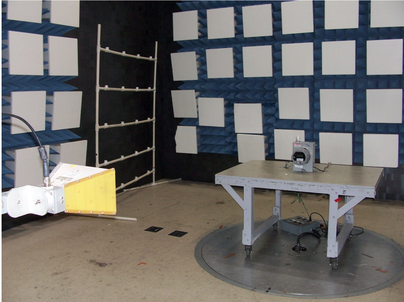
Typical View of Test Setup for Radiated Emissions from 1 GHz to 10 GHz
