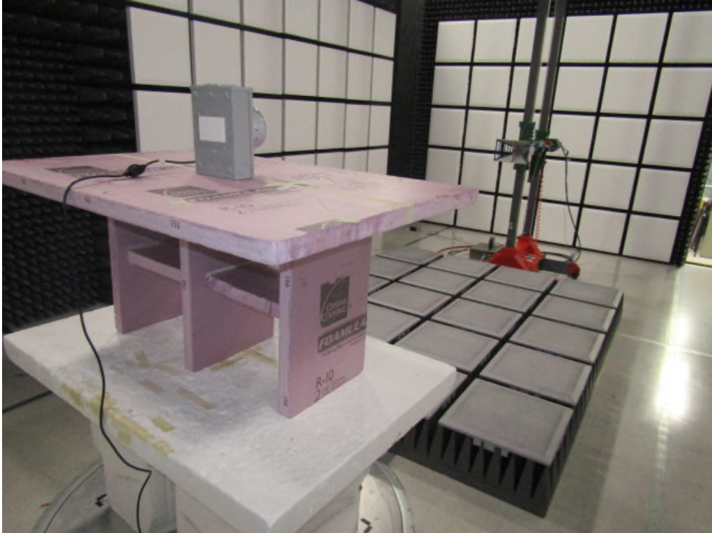
Figure 4: Radiated Emissions – Front – Above 1GHz – ZPOS
