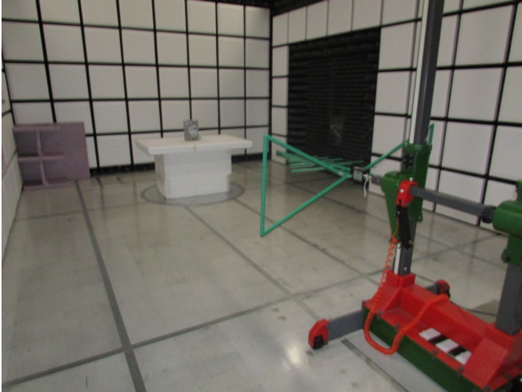
Figure 1: Radiated Emissions – Front – Below 1GHz
