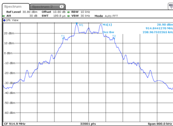
Figure 2.7.6-39: Mode 1 – 99% OBW – HCH – 38.4 kbps
