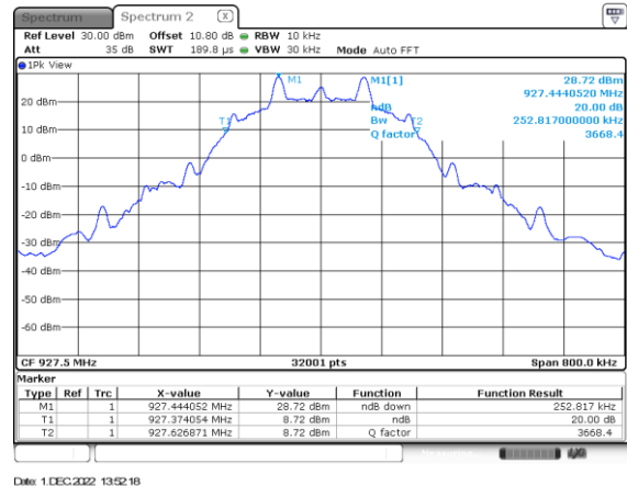
Figure 2.7.6-12: Mode 1 – 20 dB BW – HCH – 115.2 kbps
