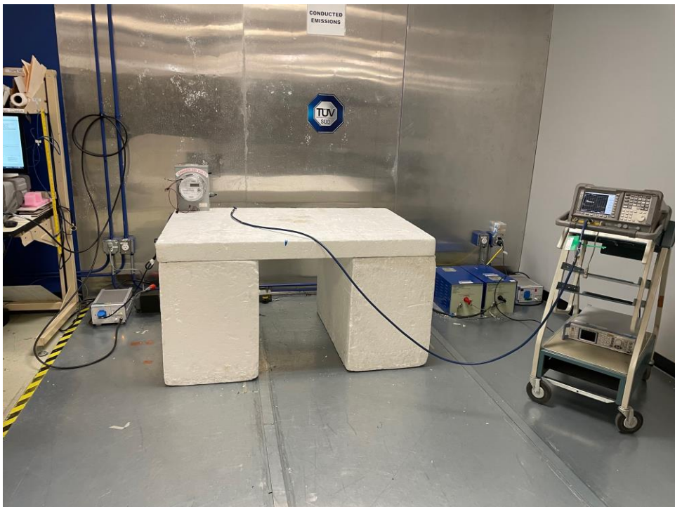
Figure4 – Test Set up – Conducted Emissions
