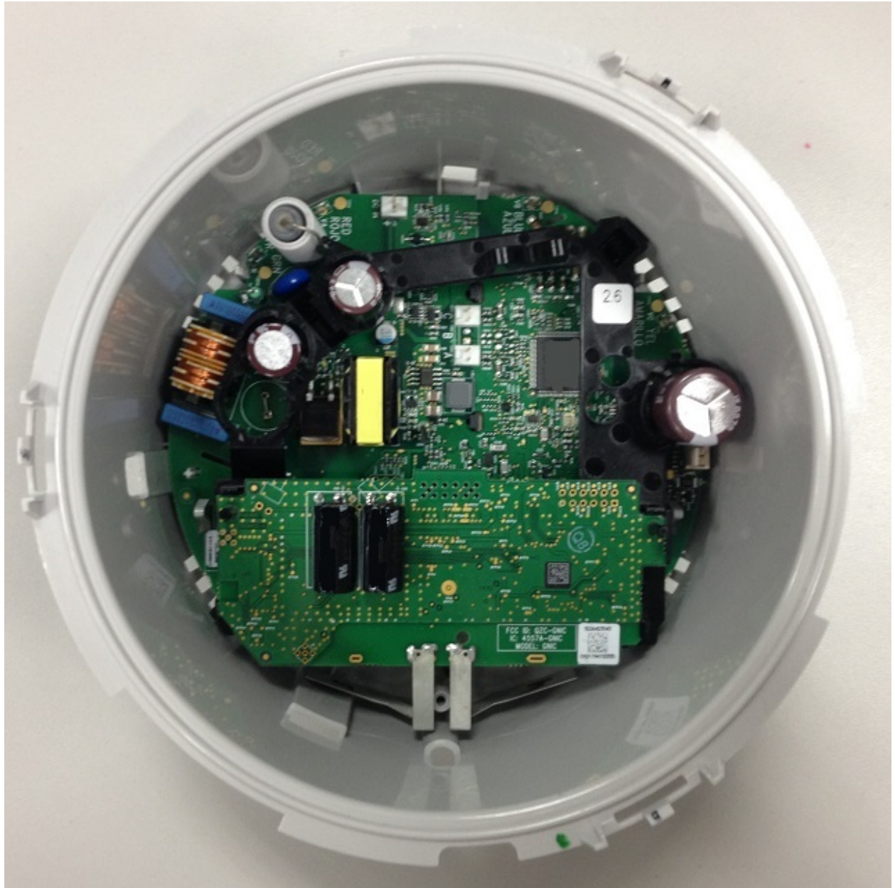
Figure 5: Module Installed in Sample Meter.
