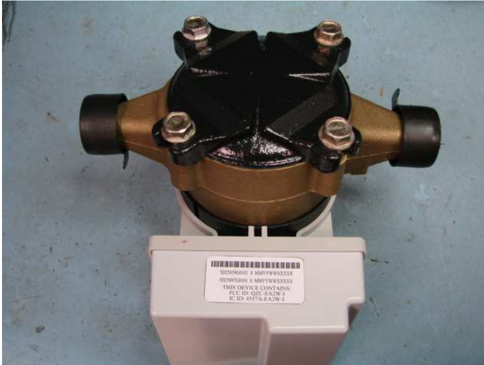
Figure 1: Location of External FCC label on EA2W-I Module, Remote Housing
