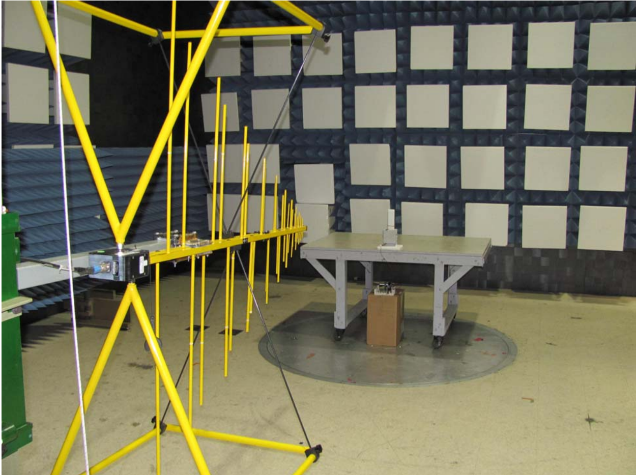
Front View of Radiated Emissions Test Setup - 30 MHz to 1 GHz
