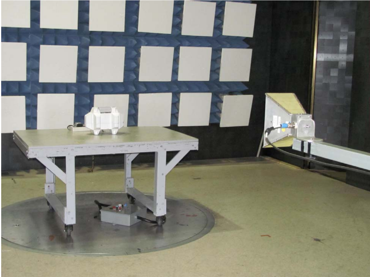
Front View of Radiated Emissions Test Setup - 1 GHz to 10 GHz
