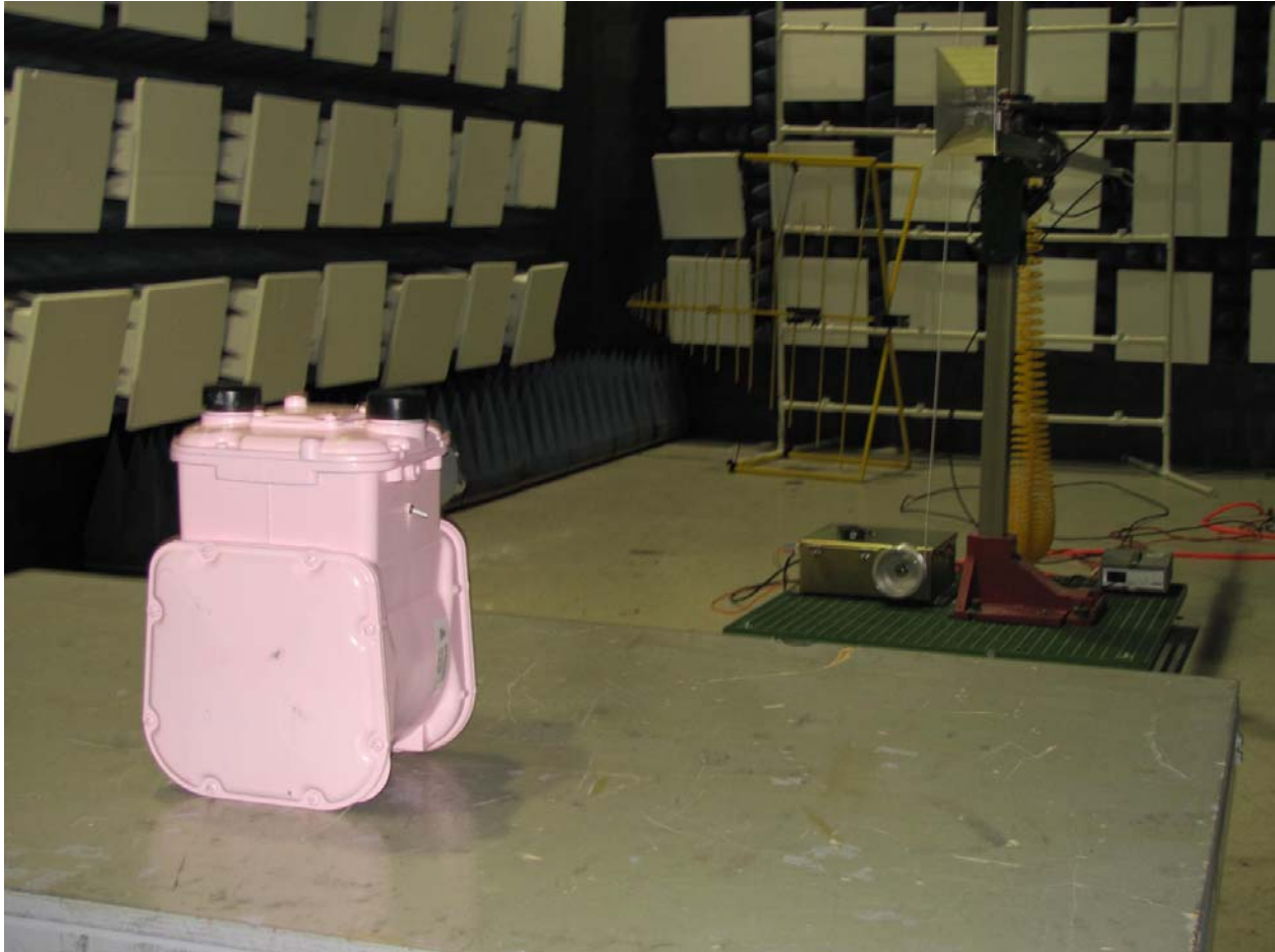
Rear View of Radiated Emissions Test Setup - 1 GHz to 10 GHz
