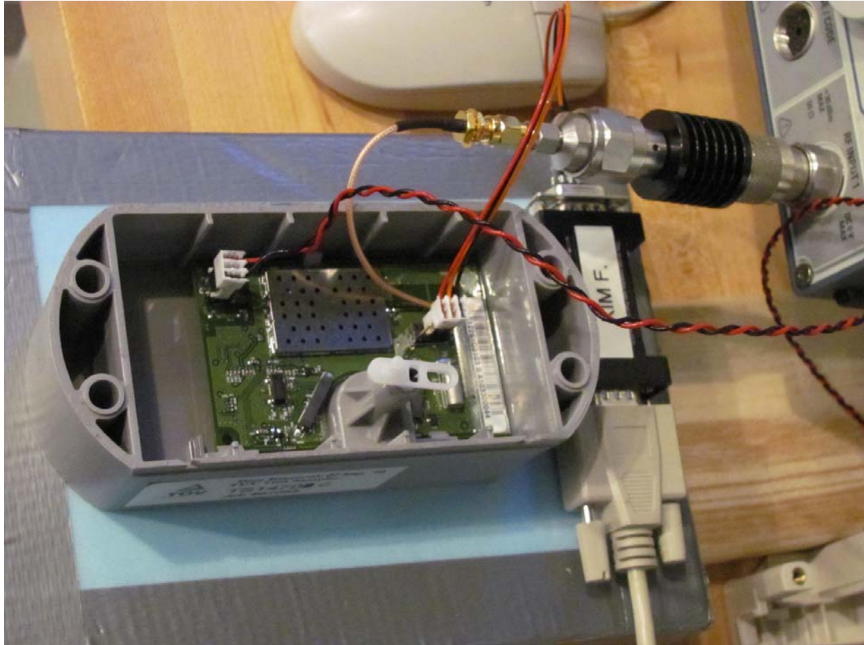
Close up View of Test Setup Making direct RF Conducted measurements
