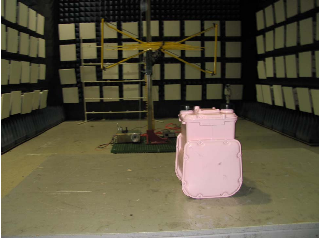
Rear View of Test Setup with the Internal Antenna - 30 MHz to 1 GHz
