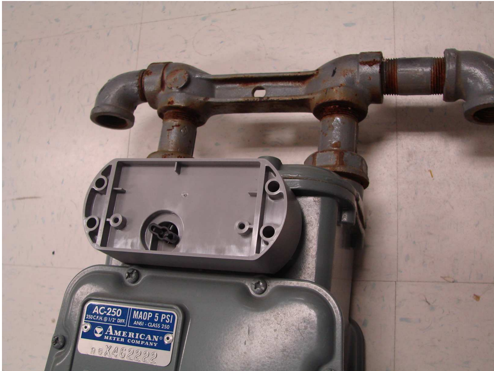
Figure 7: EA2G-I Module Partial Assembly – AMCO Gas Meter
